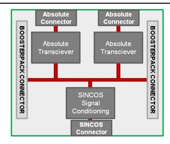
Figure 2. Position Manager BoosterPack Module Block Diagram
