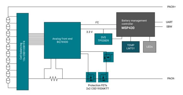
Figure 1. Block Diagram of a Li-ion Battery Pack
