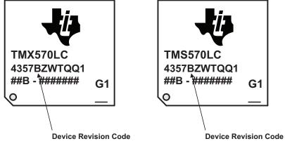
Figure 1. Device Revision Code Identification
