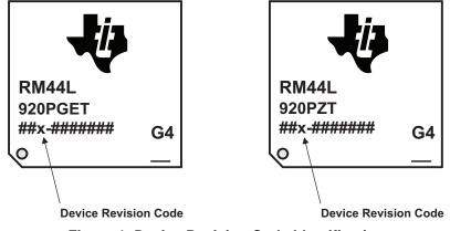
Figure 1. Device Revision Code Identification
