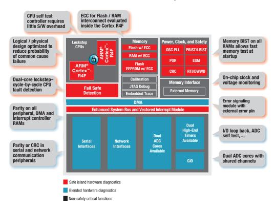
These hardware based safety features help diagnose errors in mission critical blocks and offer high diagnostic coverage with minimum software overhead.
