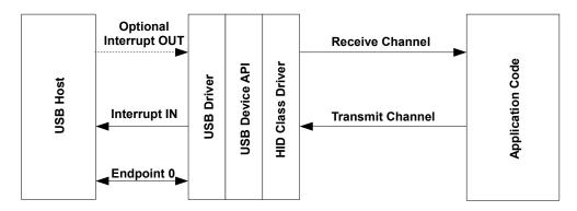
This device class uses one or, optionally, two endpoints in addition to endpoint zero. One interrupt IN endpoint carries HID input reports from the device to the host. Output and Feature reports from the host to the device are typically carried via endpoint zero but devices which expect high host-to-device data rates can select to offer an independent interrupt OUT endpoint to carry these. Endpoint zero carries standard USB requests and also HID-specific descriptor requests.
