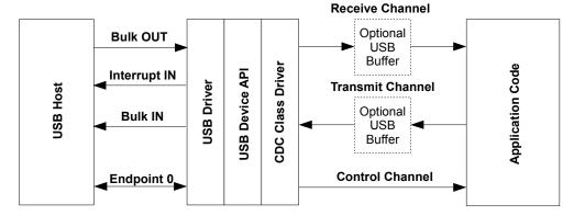
This device class uses three endpoints in addition to endpoint zero. Two bulk endpoints carry data to and from the host and an interrupt IN endpoint is used to signal any serial errors such as break, framing error or parity error detected by the device. Endpoint zero carries standard USB requests
