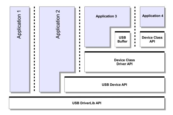
In the above diagram, bold horizontal lines represent APIs that are available for application use. Four possible applications are shown, each using a different programming interface to implement their USB functionality. The following sections provide an overview of the features and limitations of each layer and indicate the kinds of application which may choose to use that layer.
