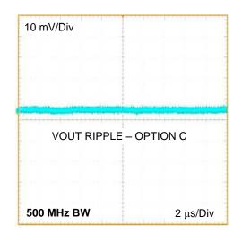
Figure 6. Output Voltage Ripple Design C  $V_{IN} = 5V$ ,  $I_{OUT} = 1A$
