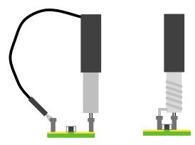
Figure 7. Oscilloscope 10X Probe
