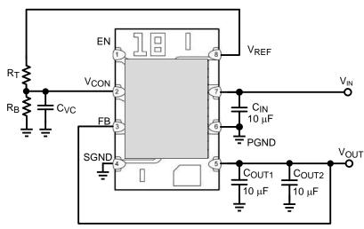
Figure 3. Schematic for Design B
