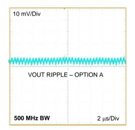
Figure 2. Output Voltage Ripple Design A  $V_{IN} = 5V, I_{OUT} = 1A$
