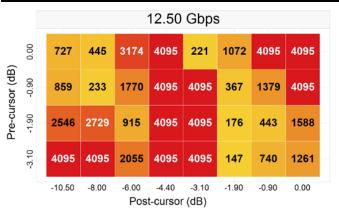
Figure 42. 35" (-36 dB) Channel No-Redriver
