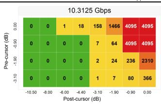
Figure 27. 15" (-14.5 dB) Pre- and 30" (-27.9 dB) Postchannel with Redriver
