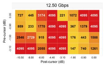
Figure 44. 35" (-36 dB) Channel No-Redriver
