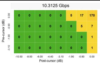
Figure 21. 25" (-22.9 dB) Pre- and 15" (-14.5 dB) Postchannel with Redriver
