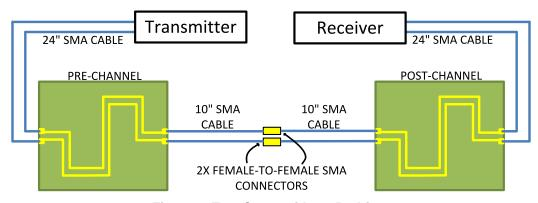
Figure 2. Test Setup without Redriver
