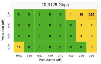
Figure 23. 35" (-31.9 dB) Pre- and 5" (-5.7 dB) Postchannel with Redriver
