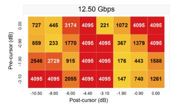
Figure 10. 35" (-36 dB) Channel No-Redriver
