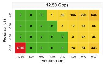
Figure 15. 10" (-11.9 dB) Pre- and 25" (-27 dB) Postchannel with Redriver
