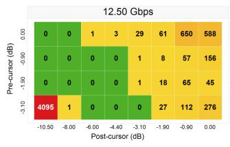
Figure 45. 25" (-27 dB) Pre- and 10" (-11.9 dB) Postchannel with Redriver
