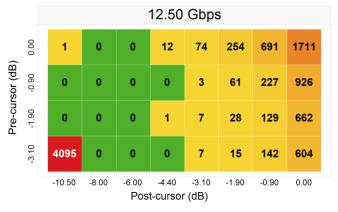
Figure 41. 5" (-6.8 dB) Pre- and 30" (-32.9 dB) Postchannel with Redriver
