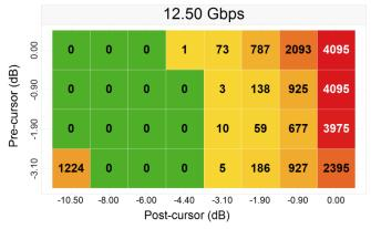
Figure 14. 30" (-31.2 dB) Channel No-Redriver
