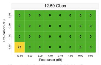
Figure 39. 25" (-27 dB) Pre- and 5" (-6.8 dB) Postchannel with Redriver
