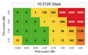
Figure 29. 30" (-27.9 dB) Pre- and 15" (-14.5 dB) Postchannel with Redriver
