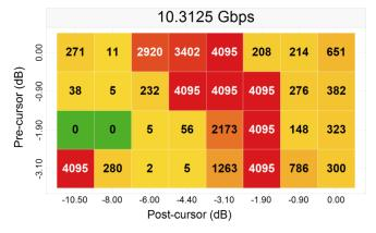
Figure 24. 45" (-38.2 dB) Channel No-Redriver
