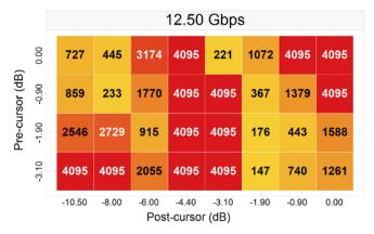
Figure 46. 35" (-36 dB) Channel No-Redriver
