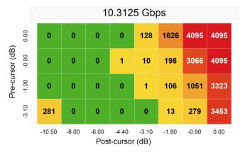
Figure 18. 40" (-33.9 dB) Channel No-Redriver
