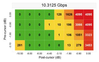
Figure 16. 40" (-33.9 dB) Channel No-Redriver
