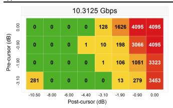
Figure 20. 40" (-33.9 dB) Channel No-Redriver
