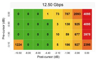
Figure 38. 30" (-31.2 dB) Channel No-Redriver
