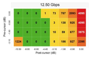
Figure 32. 30" (-31.2 dB) Channel No-Redriver
