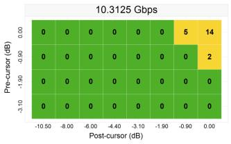
Figure 17. 5" (-5.7 dB) Pre- and 35" (-31.9 dB) Postchannel with Redriver
