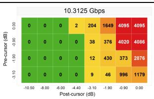
Figure 7. 5" (-5.7 dB) Pre- and 40" (-35.3 dB) Postchannel with Redriver
