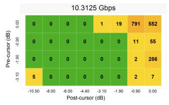
Figure 12. 35" (-30.5 dB) Channel No-Redriver
