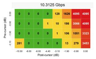
Figure 4. 40" (-33.9 dB) Channel No-Redriver
