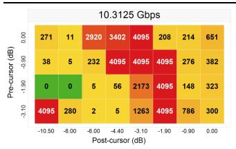
Figure 26. 45" (-38.2 dB) Channel No-Redriver
