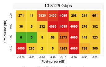
Figure 30. 45" (-38.2 dB) Channel No-Redriver
