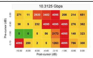
Figure 6. 45" (-38.2 dB) Channel No-Redriver
