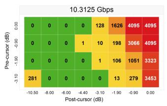
Figure 22. 40" (-33.9 dB) Channel No-Redriver
