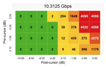
Figure 13. 5" (-5.7 dB) Pre- and 40" (-35.3 dB) Postchannel with Redriver
