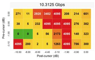
Figure 28. 45" (-38.2 dB) Channel No-Redriver
