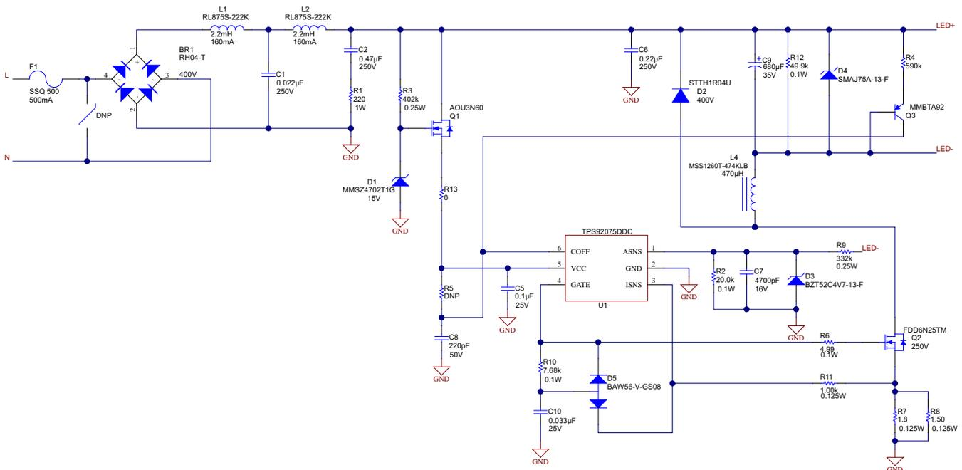
For VLED < 15 V, replace R13 with a diode (DFLS1200 or similar) and modify C5 ≥ 22 μF.
