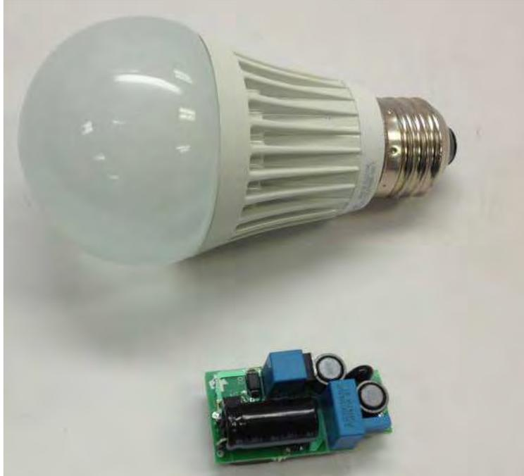
**Figure 17. EVM Board and LED Bulb**
