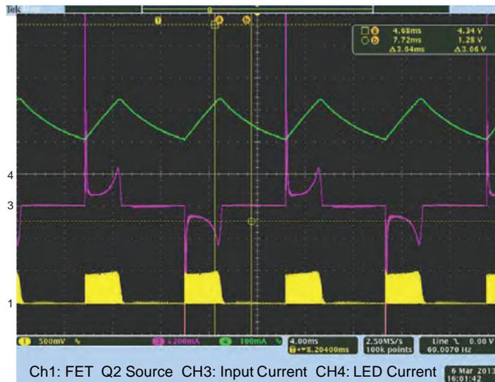
Figure 9. Lutron Leading-Edge Rotary Dimmer, Output = 150 mA,  $V_{LED} = 26\text{ V}$
