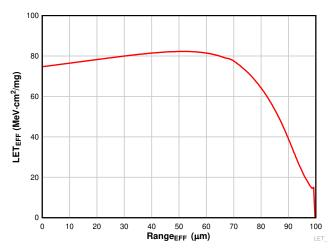
Figure 5-2. LET<sub>EFF</sub> vs Range for <sup>165</sup>Ho at the Conditions Used for the SEE Test Campaign
