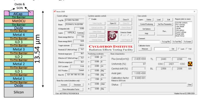
Figure 5-1. Generalized Cross Section of the BEOL Stack on the TPS7H4002A-SP [Left] and GUI of SEUSS 2020 Application Used to Determine the Ion Beam Parameters [Right]
