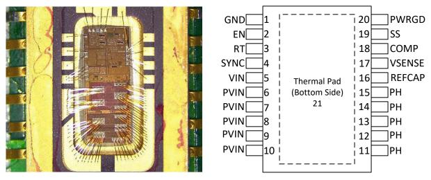
Figure 3-1. Photograph of Delidded TPS7H4002-SP [Left] and Pinout Diagram [Right]
