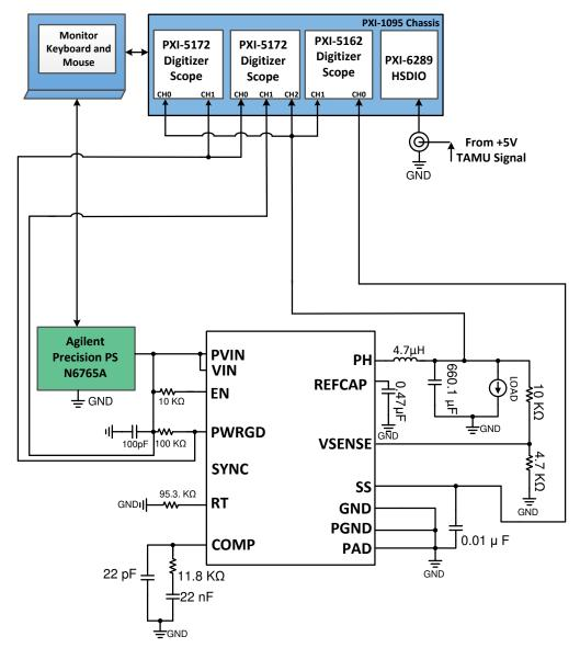
Figure 6-1. Block Diagram of SEE Test Setup for the TPS7H4002-SP
