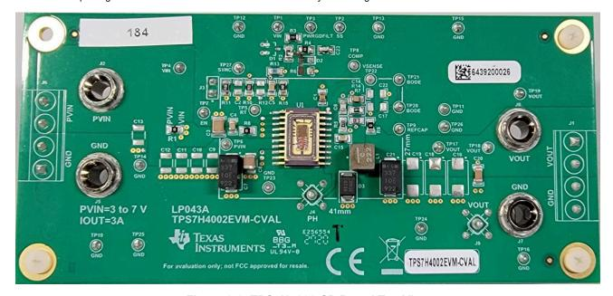
Figure 3-2. TPS7H4002-SP Board Top View
