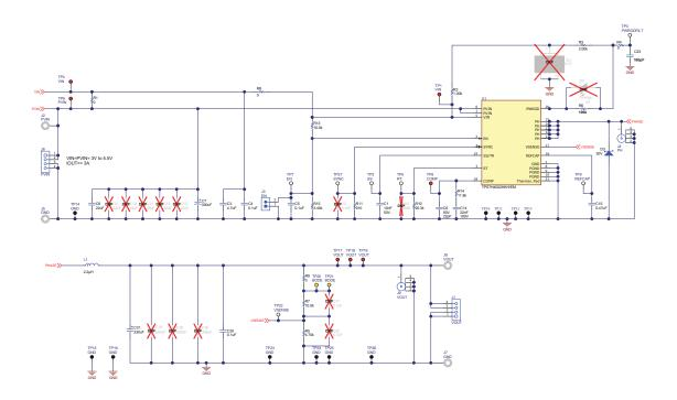
Figure 3-3. TPS7H4002EVM-CVAL Schematic
