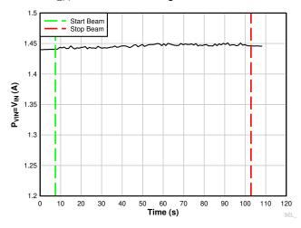
Figure 7-1. Current vs Time for Run # 2 of the TPS7H4002-SP at T = 125°C
