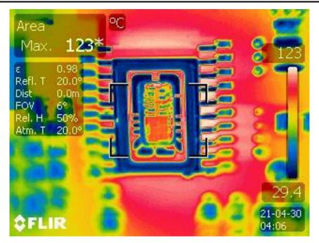
Figure 6-2. Die Temperature During the SEL Testing of the TPS7H4002-SP
