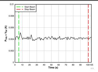
Figure 7-3. Current vs Time for Run # 6 (Disabled) for the TPS7H4002-SP at T = 25°C
