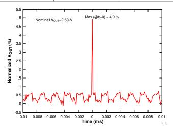
Figure 8-1. Only Observed SET  $\geq$  3% for Run # 15 at V<sub>IN</sub> = P<sub>VIN</sub> = 5 V, V<sub>OUT</sub> = 2.5 V I <sub>LOAD</sub> = 3 A and T = 25°C
