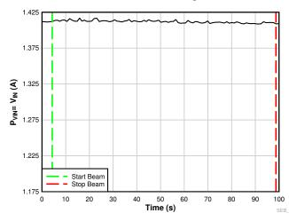
Figure 7-2. Current vs Time for Run # 5 (Enabled) for the TPS7H4002-SP at T = 25°C
