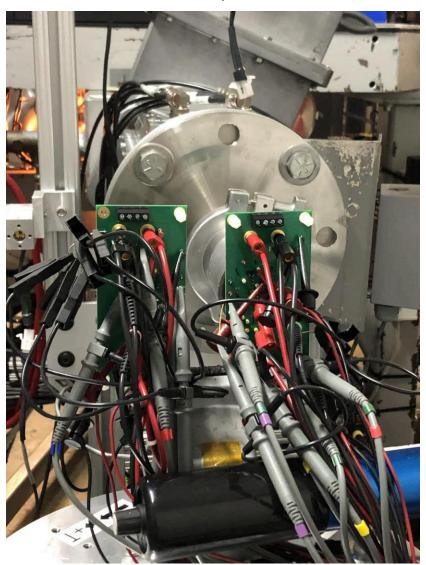
Figure 4-1. Photograph of the TPS7H4002-SP Evaluation Board Mounted in Front of the Heavy-Ion Beam Exit Port at the Texas A&M Cyclotron
