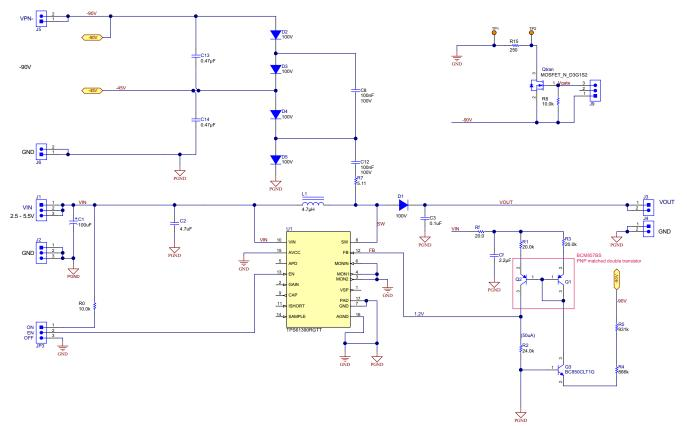
Figure 2-1. 3.3 V Input -90 V Output Conversion with TPS61391
