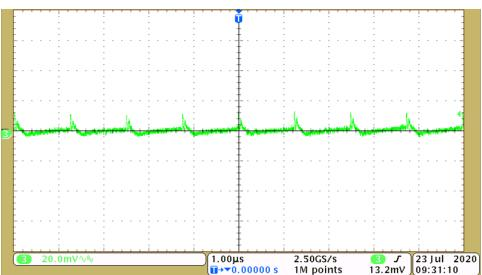
Figure 3-3. Output Voltage Ripple at 1mA load Current (Vin=3.3 V, Vout=-90 V)
