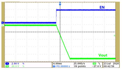
Figure 3-2. Enable Start-up Waveform (Vin=3.3 V, Vout=-90 V)
