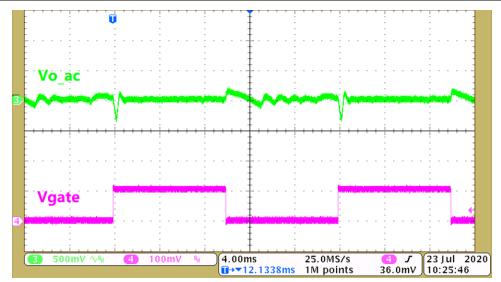
Figure 3-5. Load Dynamic Performance at 2mA Load Step (Vin=3.3 V, Vout=-90 V)
