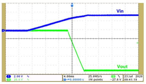
Figure 3-1. Input Voltage Start-up Waveform (Vin=3.3 V, Vout=-90 V)
