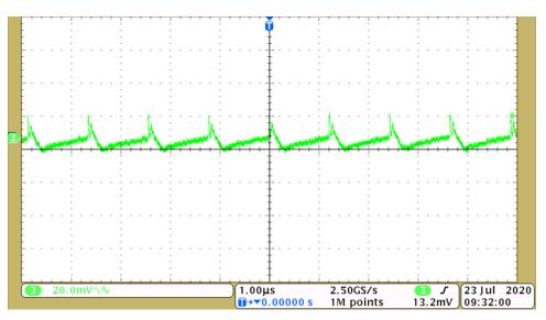
Figure 3-4. Output Voltage Ripple at 2mA load Current (Vin=3.3 V, Vout=-90 V)
