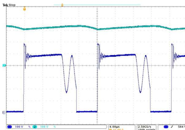
**Figure 13. Switch Node Waveform**
