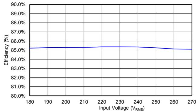
Figure 7. LM3447-PAR-230VEVM Efficiency
