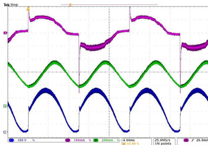
**Figure 26. Dimmer at maximum brightness setting**
