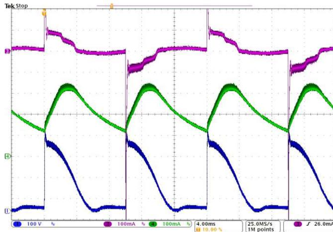
**Figure 27. Dimmer at half brightness setting**
