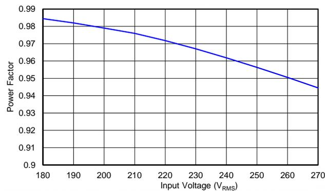
Figure 8. LM3447-PAR-230VEVM Power Factor vs Line Voltage
