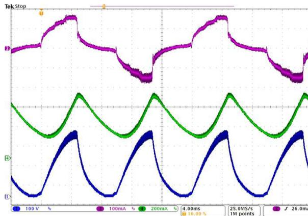
**Figure 23. Dimmer at half brightness setting**
