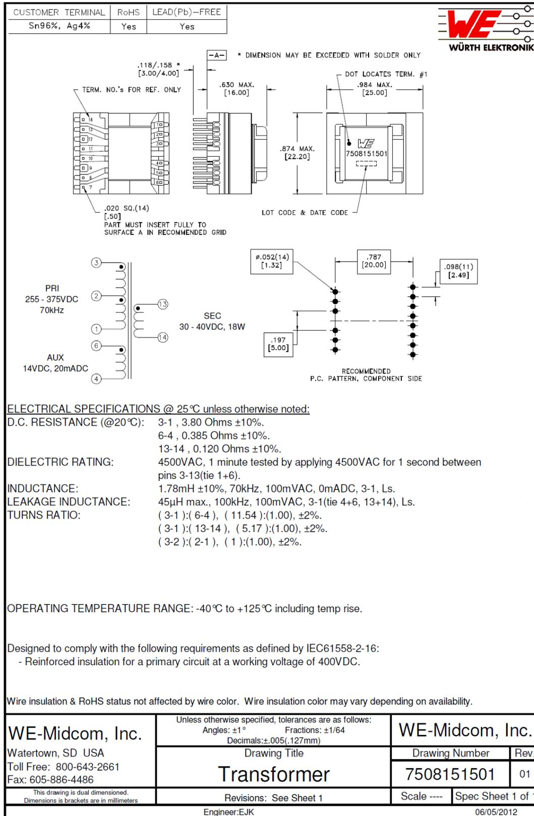
**Figure 33. Transformer Specification**
