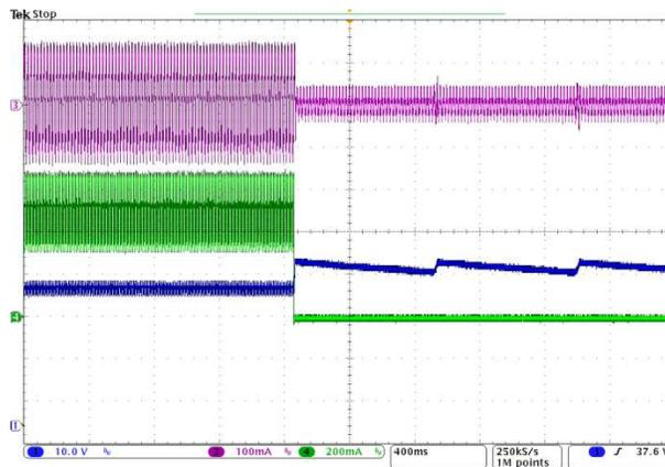
**Figure 17. Open Circuit Transient Waveforms**
