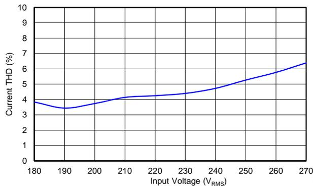
Figure 11. LM3447-PAR-230VEVM- Current THD % vs Line Voltage
