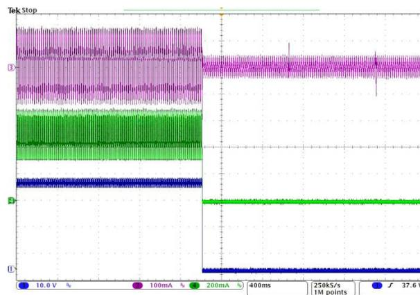
**Figure 20. Short Circuit Transient Waveforms**
