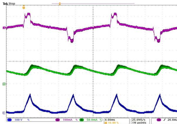
**Figure 24. Dimmer at minimum brightness setting**
