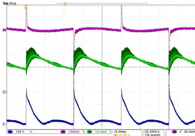
**Figure 28. Dimmer at minimum brightness setting**
