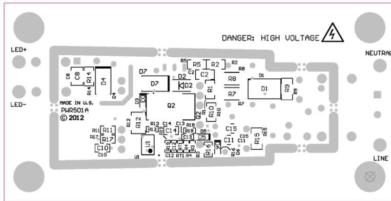
Figure 6. LM3447-PAR-230VEVM Bottom Assembly Drawing (bottom view)
