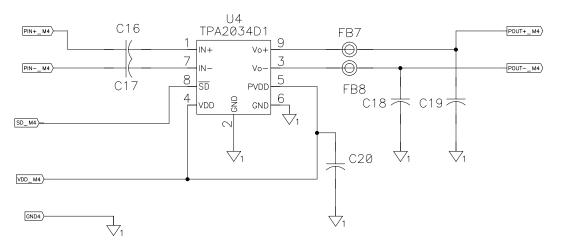
Figure 7. TPA2032xD1 Mini EVM Schematic Diagrams
