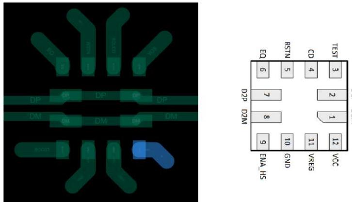
Figure 2. Flow-through Design
