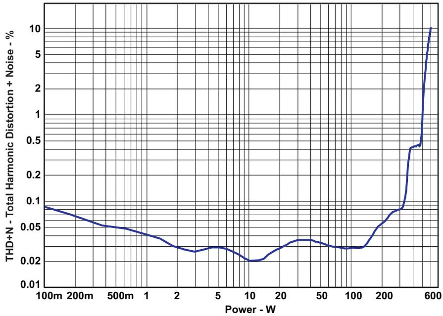
Figure 6. THD+N vs Power (PBTL -2 Ω)
