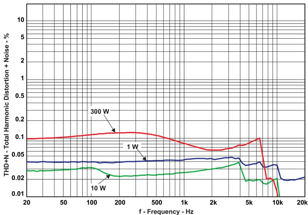
Figure 9. THD+N vs Frequency (PBTL –2 Ω)
