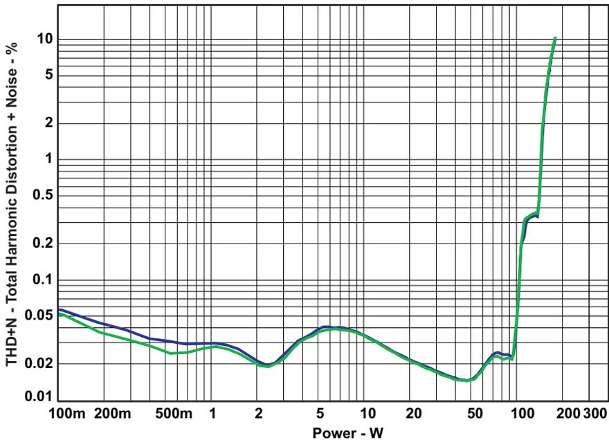
Figure 5. THD+N vs Power (BTL –8 Ω)
