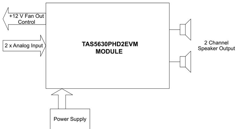
**Figure 1. Integrated PurePath™ Premier Pro Amplifier System**
