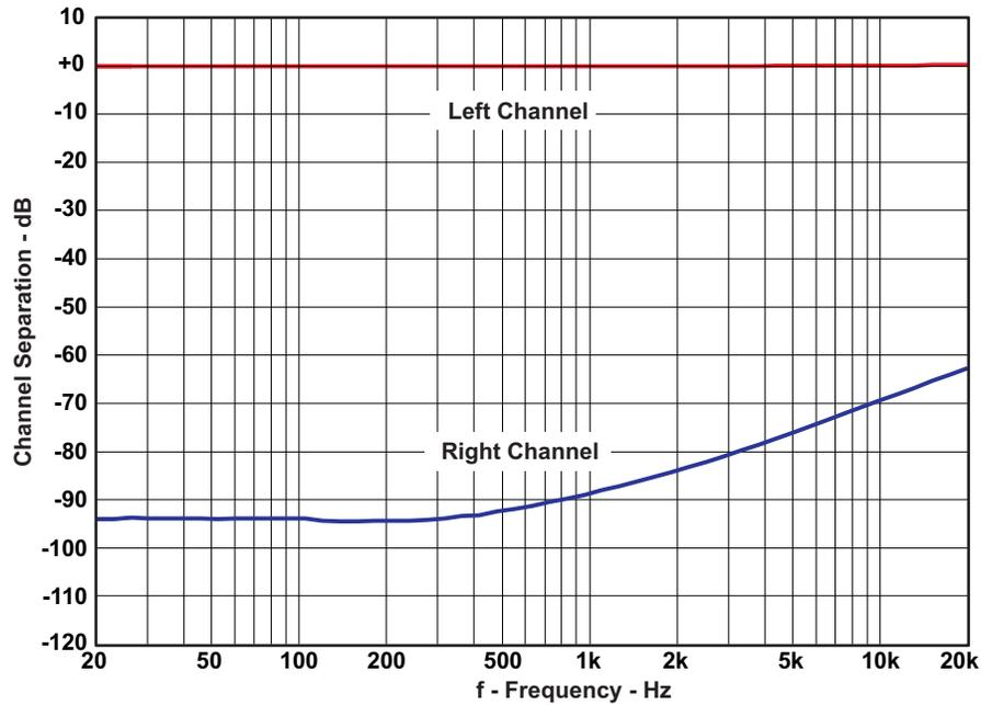
Figure 14. Channel Separation
