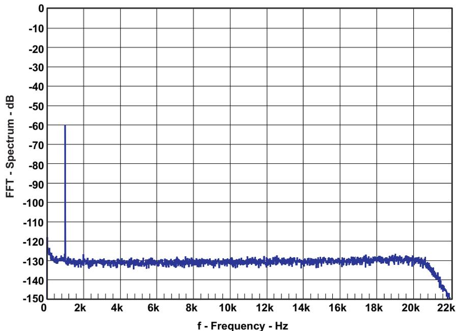
Figure 11. FFT Spectrum with -60-dBFS Tone (PBTl)
