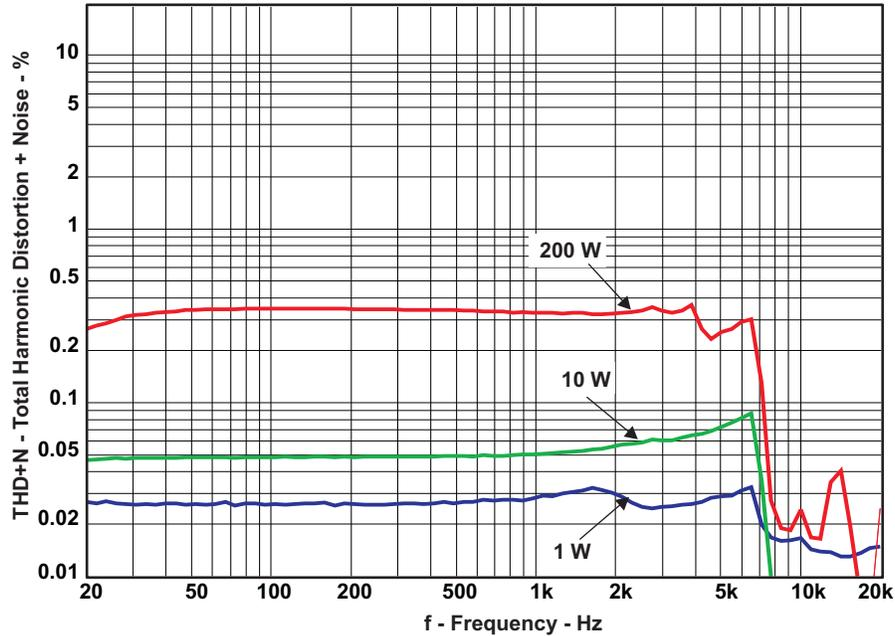
Figure 7. THD+N vs Frequency (BTL -4 Ω)
