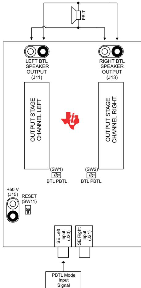
**Figure 2. Physical Structure for the TAS5630PHD2EVM (Approximate Layout)**
