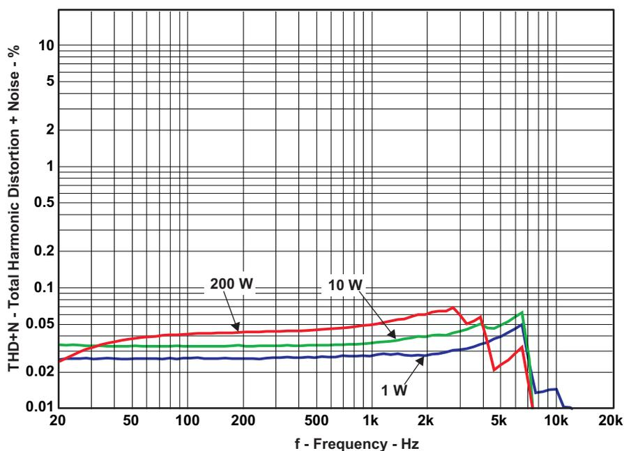
Figure 8. THD+N vs Frequency (BTL –8 Ω)
