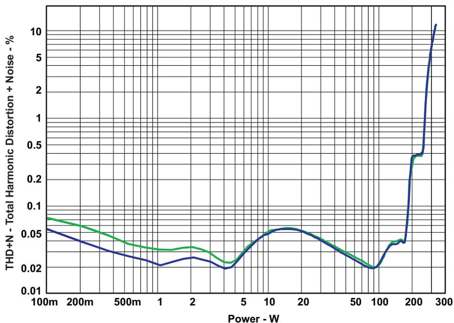
Figure 4. THD+N vs Power (BTL –4 Ω)
