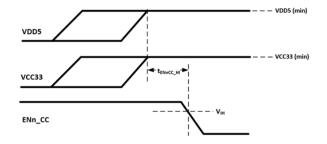
Figure 4-3. Power On Sequence of HD3SS3220 With ENn\_CC
