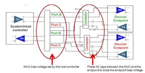
Figure 7-1. AC Capacitor Placed at Endpoint Side
