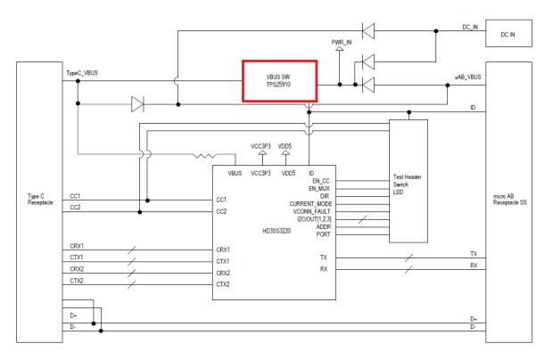
Figure 6-1. DFP Application With VBUS Switch
