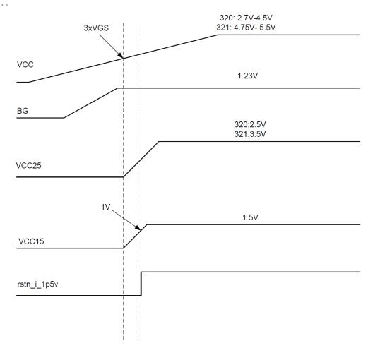
Figure 4-1. Power On Reset Timing of TUSB32x Devices
