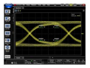
Figure 3-7. Output Waveform after 1st Multiplexer
