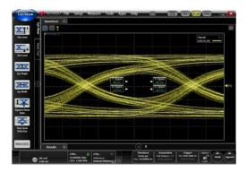
Figure 3-8. Output Waveform after 2nd Multiplexer
