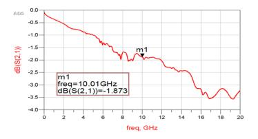
Figure 3-2. Insertion Loss of TMUXHS4212
