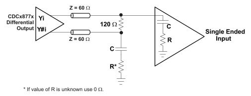
Figure 4. Example Termination for Differential Signal That Drives a Single-Ended Input Stage
