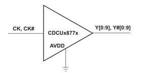
Figure 2. The CDCUx877x Used as 1:10 Clock Buffer
