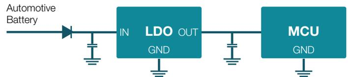
Figure 9: Automotive battery-direct-connect LDO simplified application diagram.
