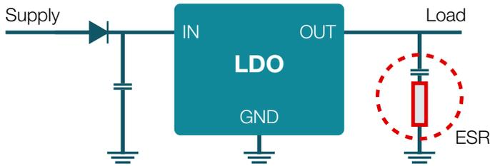
**Figure 29:** Output capacitor and ESR.
