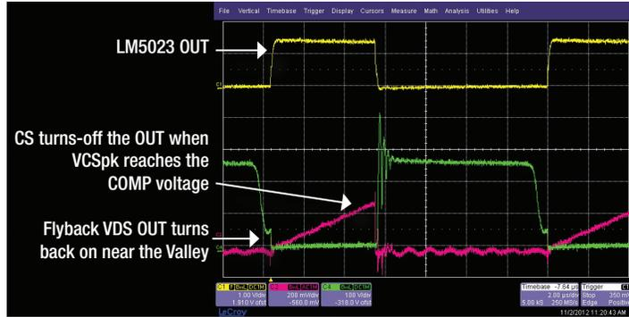
Figure 2. Typical QR switching waveforms
