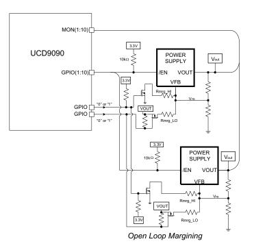
Figure 21. Open-Loop Margining
