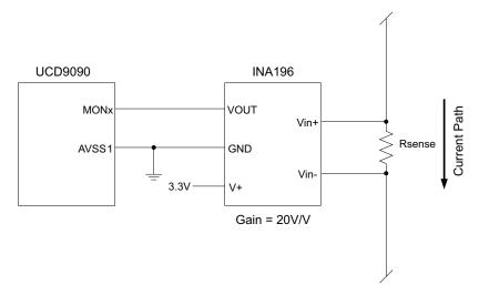
Figure 11. Current Monitoring Circuit Example Using the INA196
