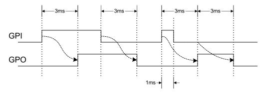
Figure 19. GPO Behavior When Ignoring Inputs During Delay
