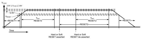
Figure 28. UCD9090-Q1 RESET1 and RESET2 Behavior
