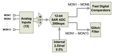
Figure 10. Voltage Monitoring Block Diagram
