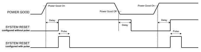
Figure 23. System Reset With and Without Pulse Setting
