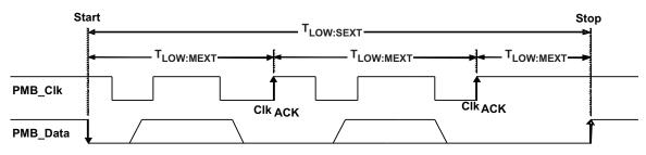
Figure 2. Bus Timing in Extended Mode
