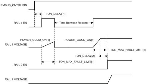
Rail 1 and Rail 2 are both sequenced "ON" and "OFF" by the PMBUS\_CNTRL pin only
