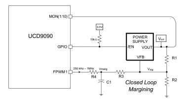
Figure 22. Closed-Loop Margining
