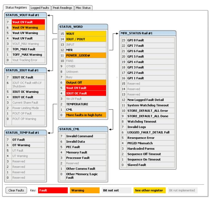
Figure 7. Fusion GUI Rail-Status Register
