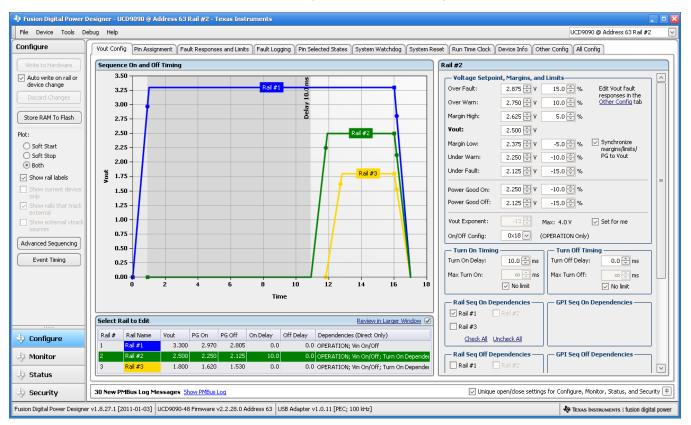
Figure 5. Fusion GUI V<sub>OUT</sub>-Config Tab
