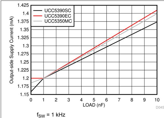
图 6-23.  $I_{CC2}$  Supply Current vs Load Capacitance
