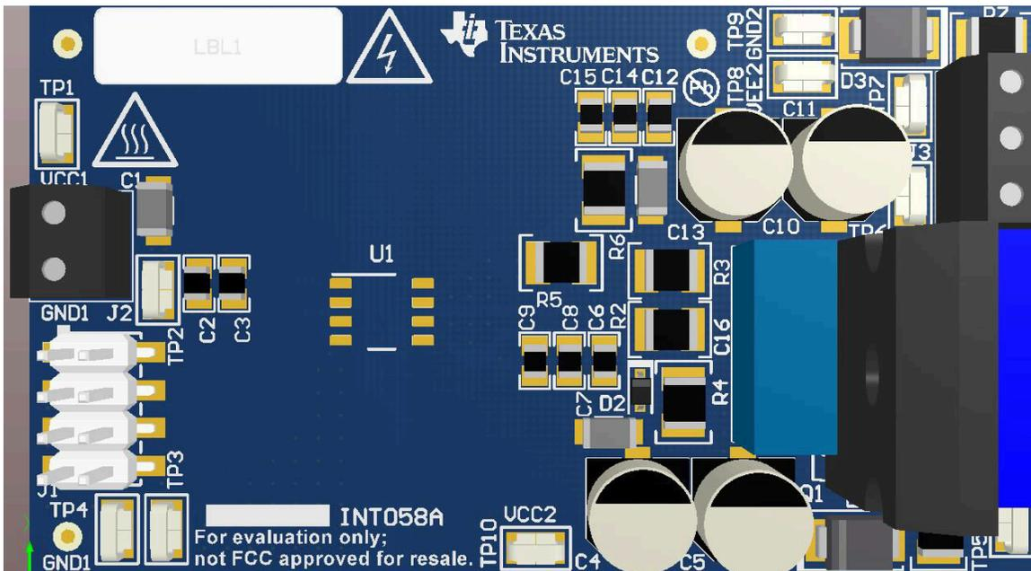
A. The location of the PCB cutout between primary side and secondary sides ensures isolation performance.
