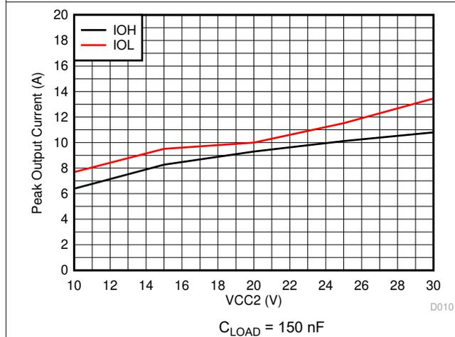
图 6-7. UCC5350SBD Output-High Drive Current vs Output Voltage
