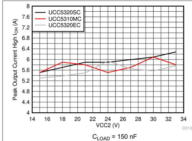
图 6-5. Output-High Drive Current vs Output Voltage
