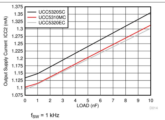
图 6-22.  $I_{CC2}$  Supply Current vs Load Capacitance
