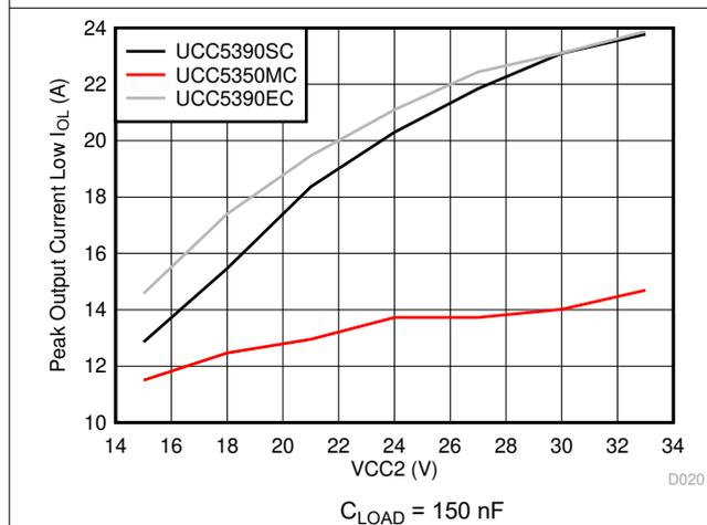
图 6-9. Output-Low Drive Current vs Output Voltage
