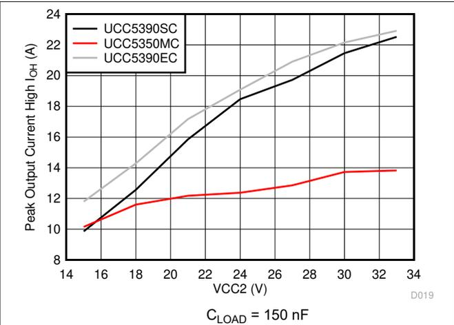
图 6-6. Output-High Drive Current vs Output Voltage
