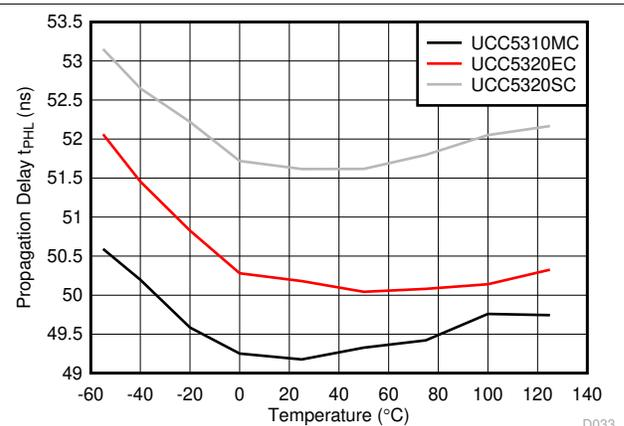
图 6-34. Propagation Delay  $t_{PHL}$  vs Temperature
