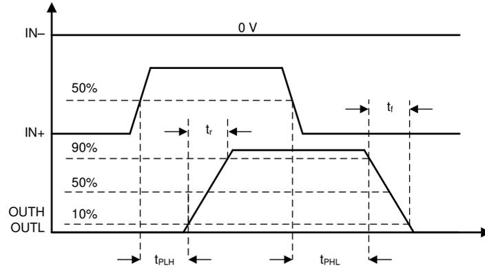
图 7-1. OUTH and OUTL Propagation Delay, Noninverting Configuration
