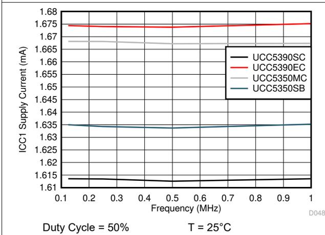
图 6-15.  $I_{CC1}$  Supply Current vs Input Frequency
