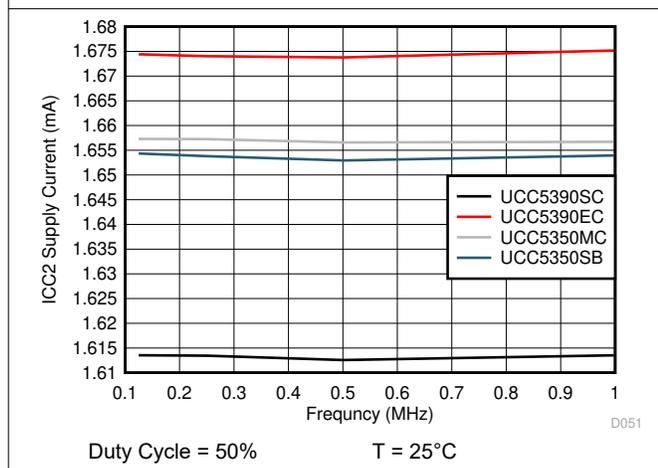
图 6-21.  $I_{CC2}$  Supply Current vs Input Frequency
