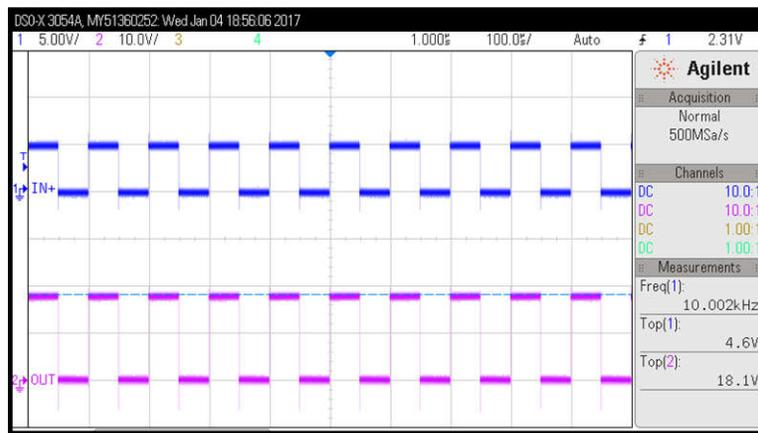
$V_{CC2} = 20\text{ V}$        $V_{EE2} = \text{GND}$        $f_{\text{SW}} = 10\text{ kHz}$
