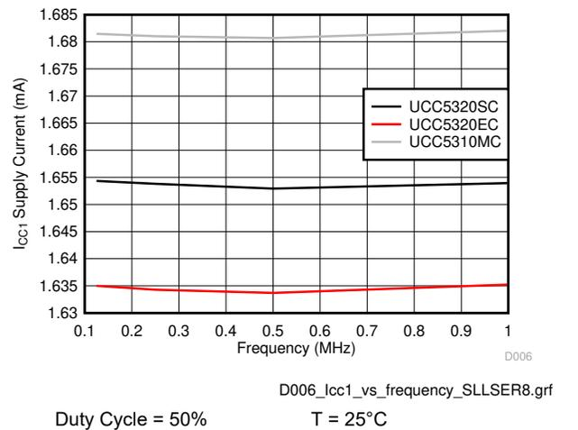
图 6-14.  $I_{CC1}$  Supply Current vs Input Frequency
