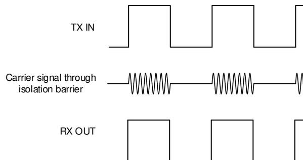
图 8-2. On-Off Keying (OOK) Based Modulation Scheme
