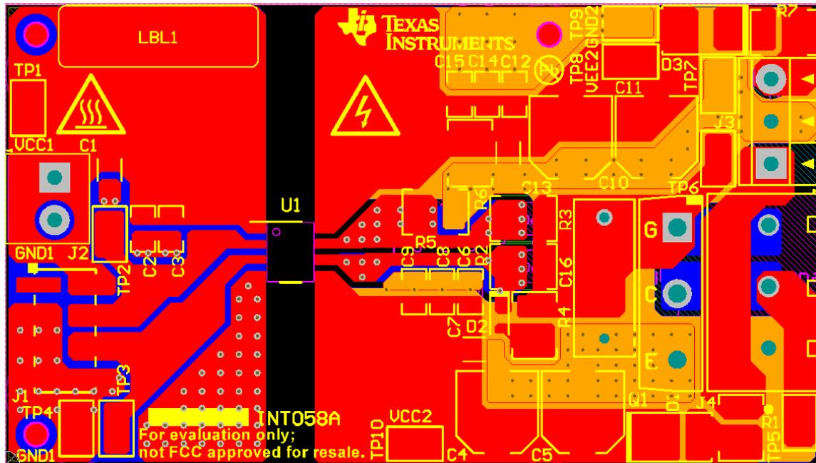
A. No PCB traces or copper are located between the primary and secondary side, which ensures isolation performance.
