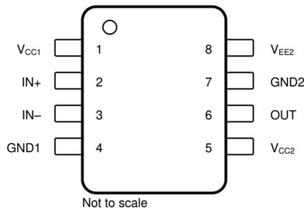
图 5-3. UCC5320E and UCC5390E 8-Pin SOIC Top View
