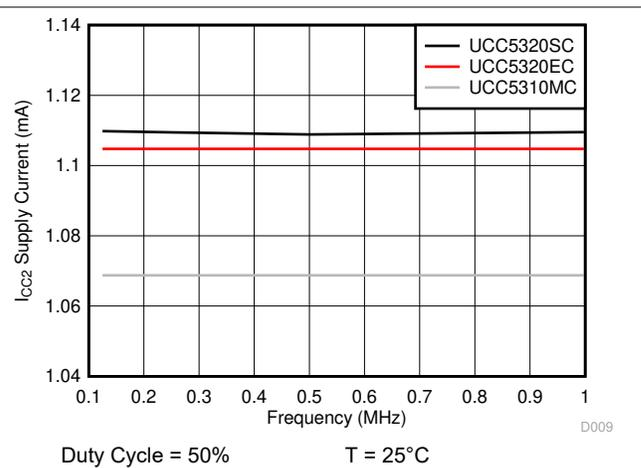
图 6-20.  $I_{CC2}$  Supply Current vs Input Frequency
