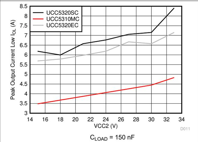
图 6-8. Output-Low Drive Current vs Output Voltage
