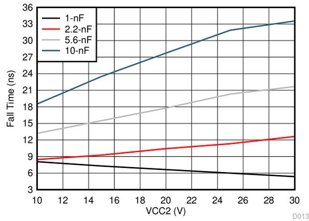
图 6-41. UCC5350SBD Fall Time vs  $C_L$  and  $V_{CC2}$
