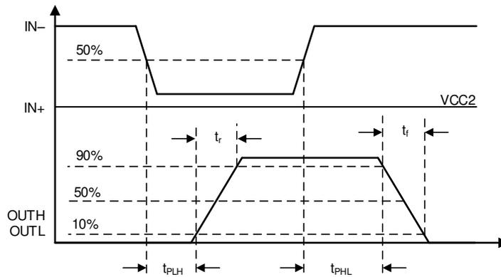
图 7-2. OUTH and OUTL Propagation Delay, Inverting Configuration
