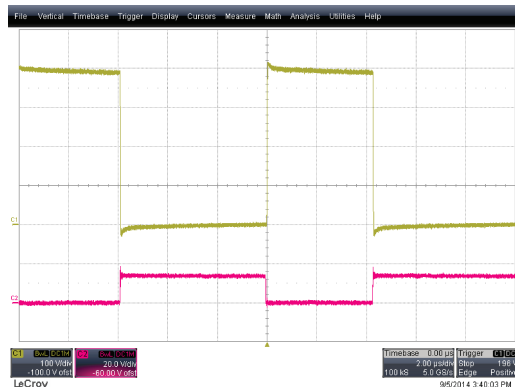
Figure 42. PFC Stage Switching (C1: V DS , C2: PFC_GD See Figure 34 )
