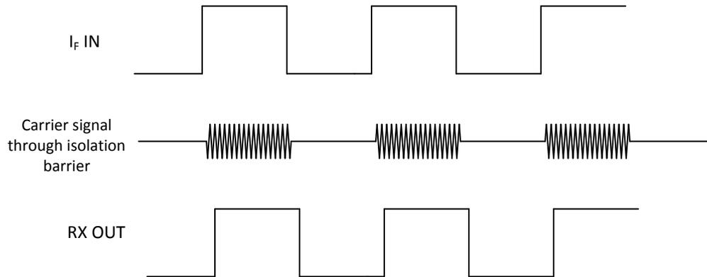
**图 8-2. On-Off Keying (OOK) Based Modulation Scheme**
