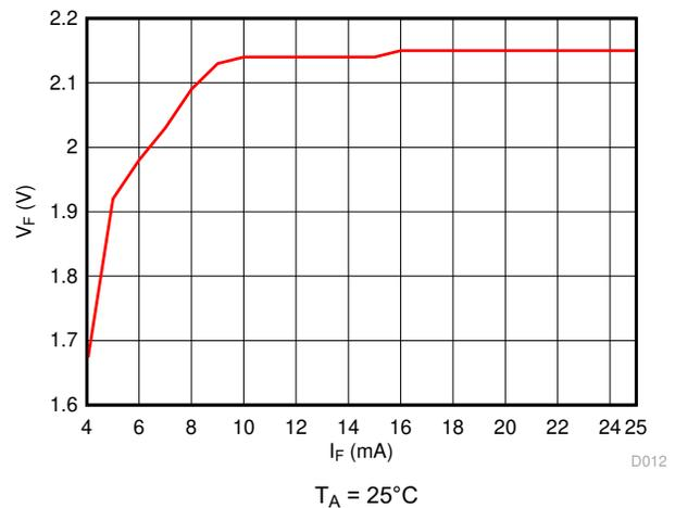
图 6-12. Forward Current vs Forward Voltage Drop
