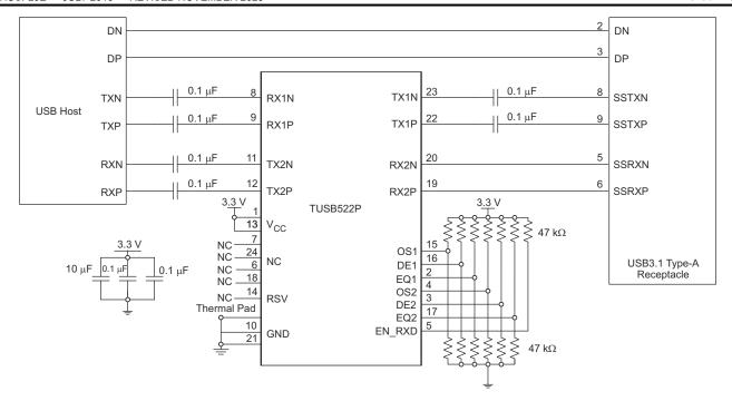
图 8-2. Embedded Host Application Schematic
