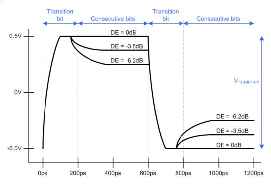
图 7-1. Transmitter Differential Voltage, OS = Floating
