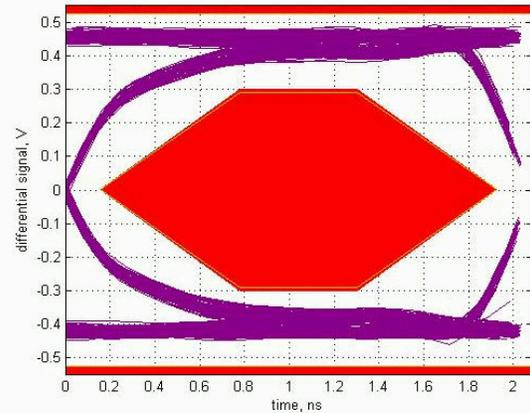
图 9-5. HighSpeed TX Eye for Downstream Port 2
