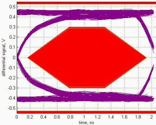
图 9-4. HighSpeed TX Eye for Downstream Port 1
