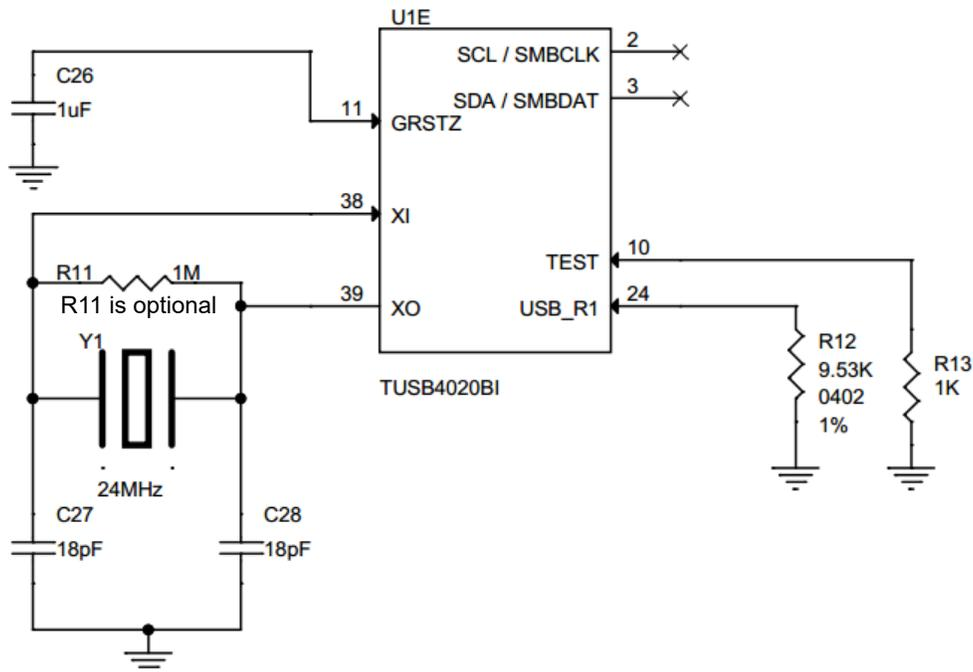
图 9-9. Clock, Reset, and Miscellaneous Schematic
