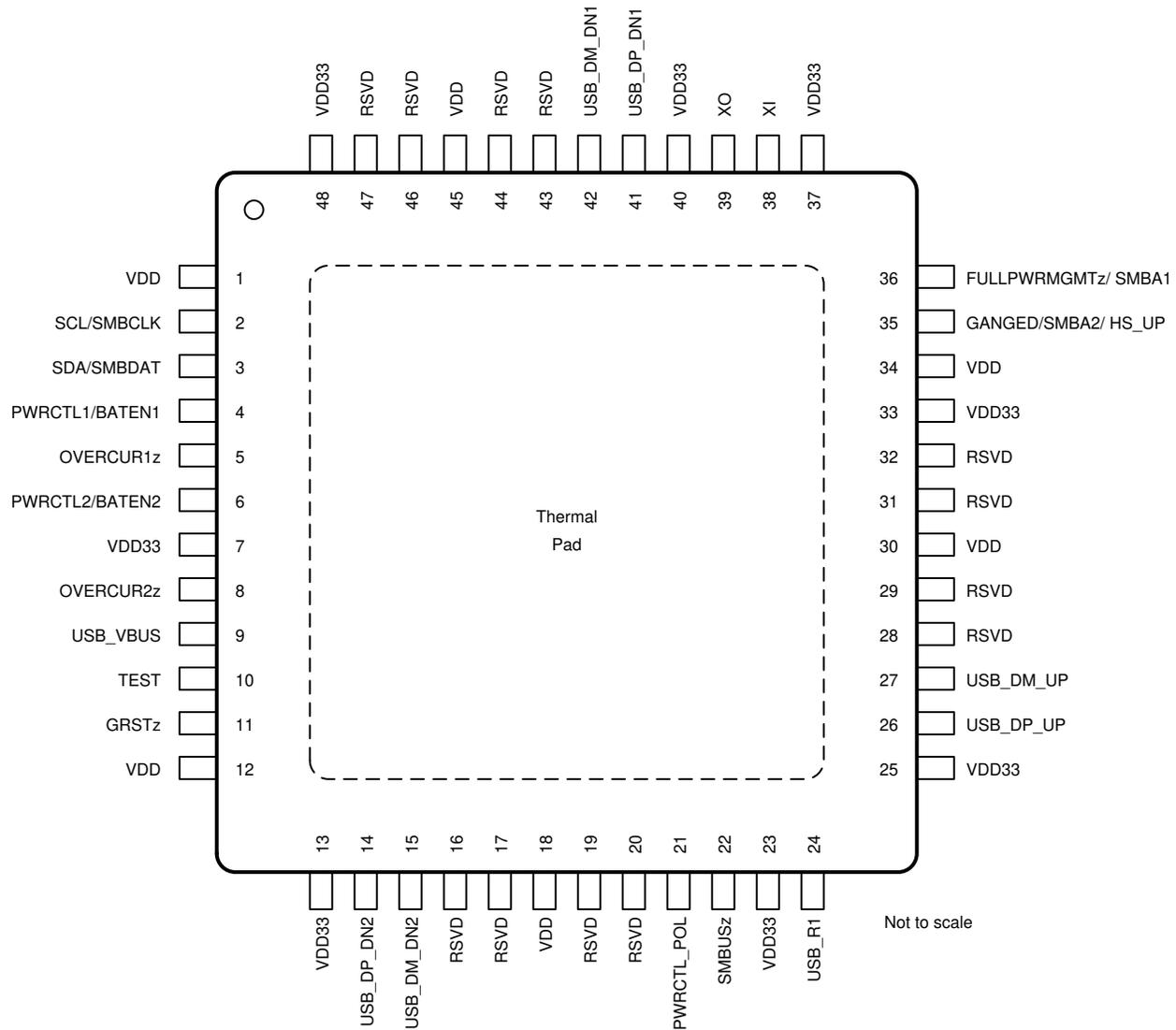
图 6-1. PHP Package 48-Pin HTQFP Top View
