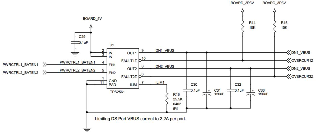
图 9-8. Power Switch Implementation Schematic
