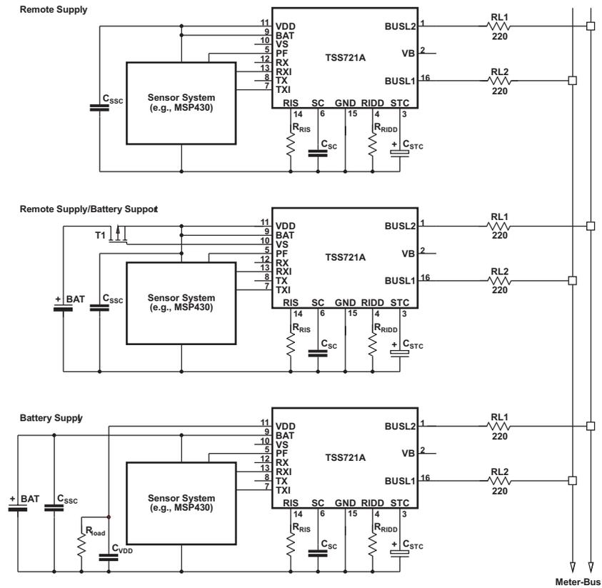
NOTE:  $R_{DSon}$  of the transistor T1 (BSS84) at low battery voltage must be considered during application design.
