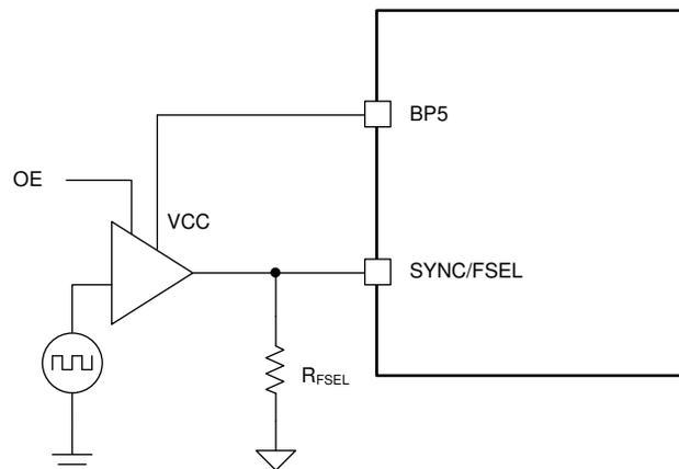
图 6-5. Interfacing the SYNC/FSEL Pin With a Buffer
