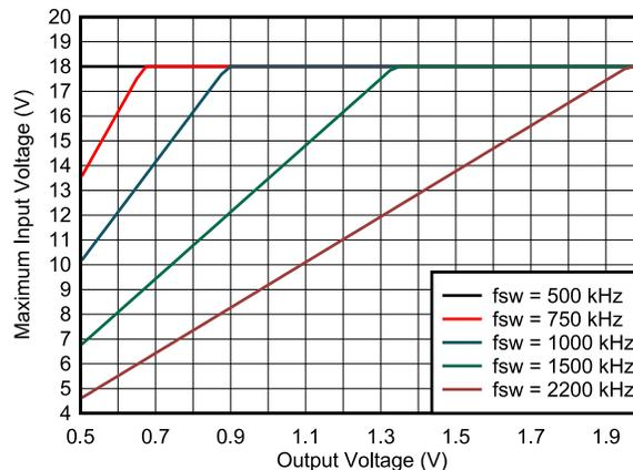
图 7-2. Maximum Input Voltage vs Output Voltage
