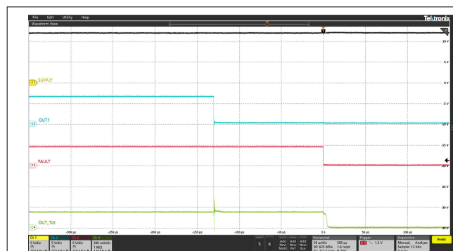
图 6-13. LED Short-Circuit Protection
