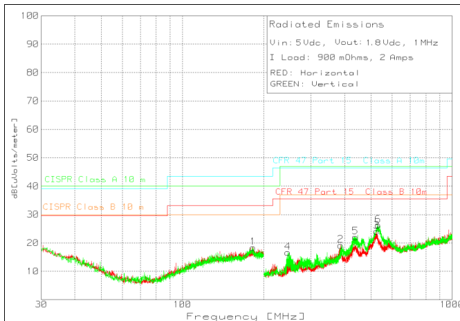
Figure 36. Radiated Emissions 5-V Input, 1.8-V Output, 2-A Load (EN55022 Class B)
