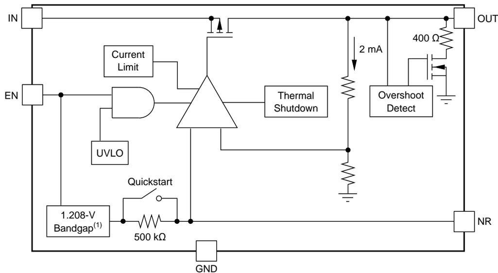
NOTE: Fixed voltage versions between 1 V to 1.2 V have a 1-V band-gap circuit instead of a 1.208-V band-gap circuit.
