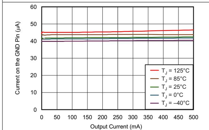
Figure 5. TPS73525-Q1 Ground Pin Current vs Output Current
