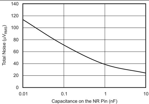
Figure 11. TPS73525-Q1 RMS Noise vs  $C_{NR}$
