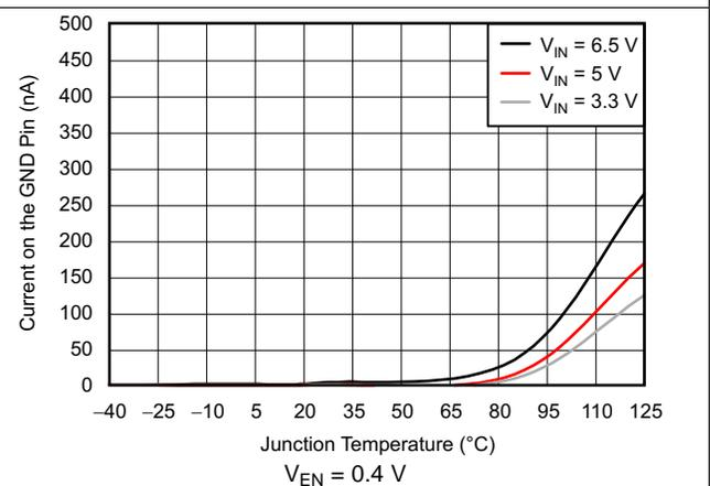
Figure 6. TPS73525-Q1 Ground Pin Current (Disable) vs Temperature
