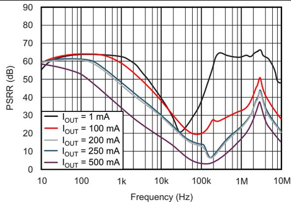
Figure 10. Power-Supply Ripple Rejection vs Frequency ( $V_{IN} - V_{OUT} = 0.3\text{ V}$ )
