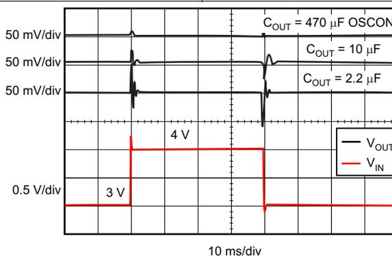
Figure 21. TPS73525-Q1 Line Transient Response
