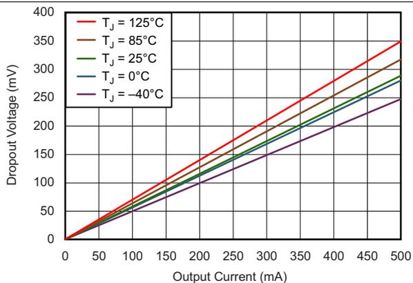
Figure 7. TPS73501-Q1 Dropout Voltage vs Output Current
