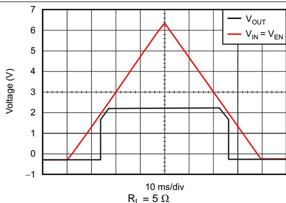
Figure 19. TPS73525-Q1 Power-Up and Power-Down ( $V_{IN} = V_{EN}$ )
