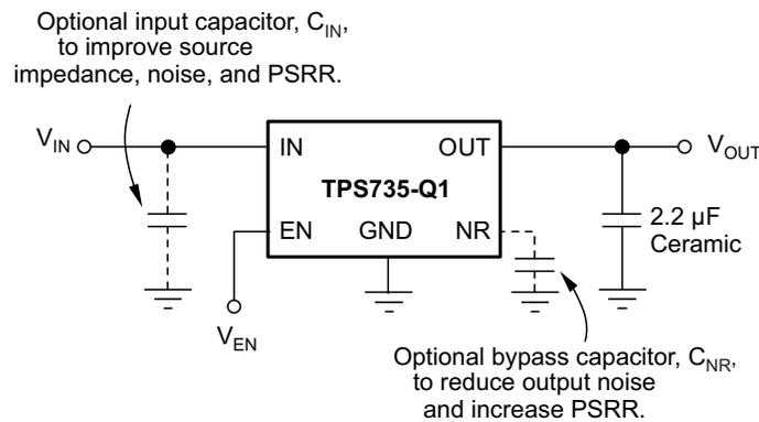
Figure 15. Typical Application Circuit for Fixed Voltage Versions
