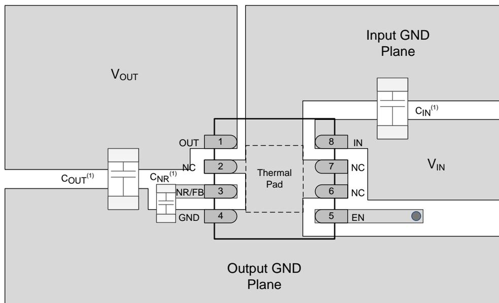
(1)  $C_{IN}$  and  $C_{OUT}$  are 0603 capacitors and  $C_{NR}$  is a 0402 capacitor. The footprint is shown to scale with package size.
