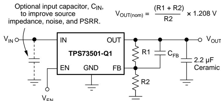
Figure 16. Typical Application Circuit for Adjustable Voltage Versions
