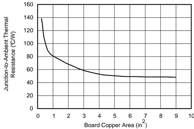
NOTE: The  $R_{\theta JA}$  value at a board size of 9 in<sup>2</sup> (that is, 3 in × 3 in) is a JEDEC standard.
