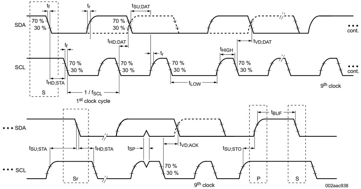
图 7-1. I<sup>2</sup>C Slave Interface Timing
