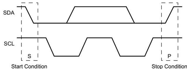
图 8-23. I<sup>2</sup>C Definition of Start and Stop Conditions
