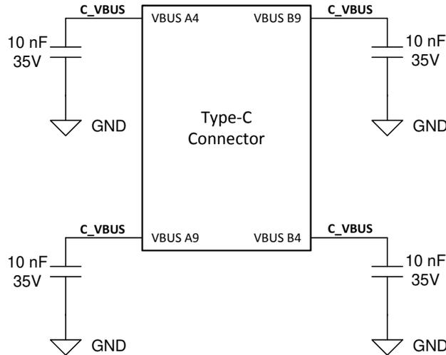
图 9-2. Type-C Connector VBUS Capacitors
