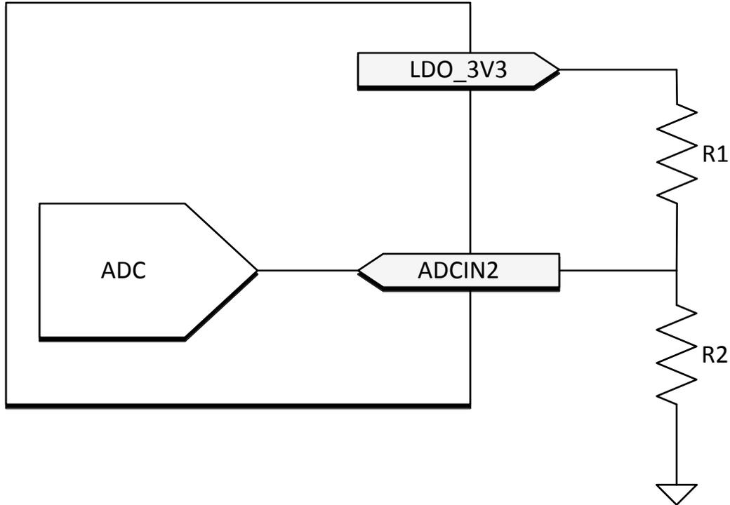
图 8-29. I<sup>2</sup>C Address Divider
