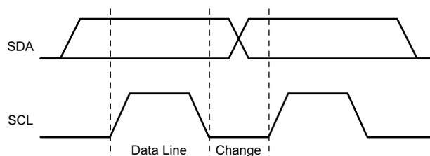
图 8-24. I<sup>2</sup>C Bit Transfer
