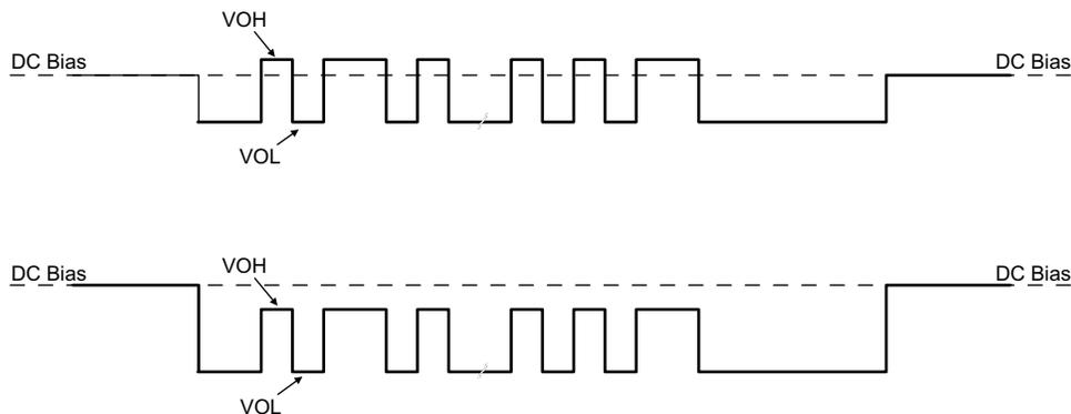
图 8-6. TX Driver Transmission with DC Bias
