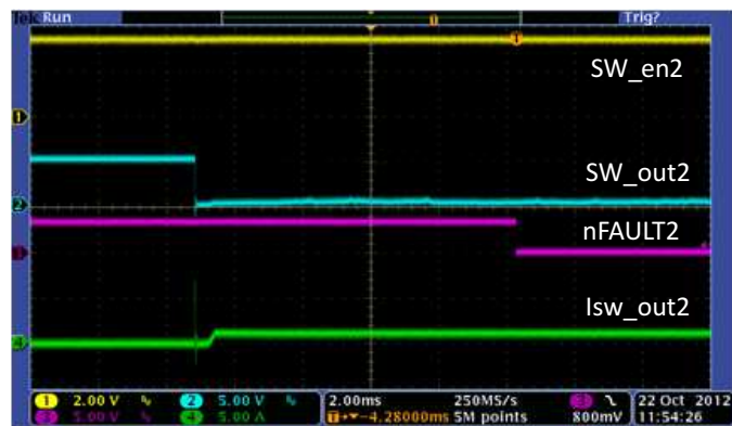
Figure 42. USB Switch2 Current Limit Operation
