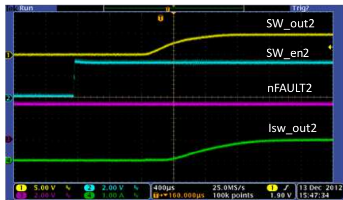
Figure 40. USB Switch2 Start-Up 1A Load
