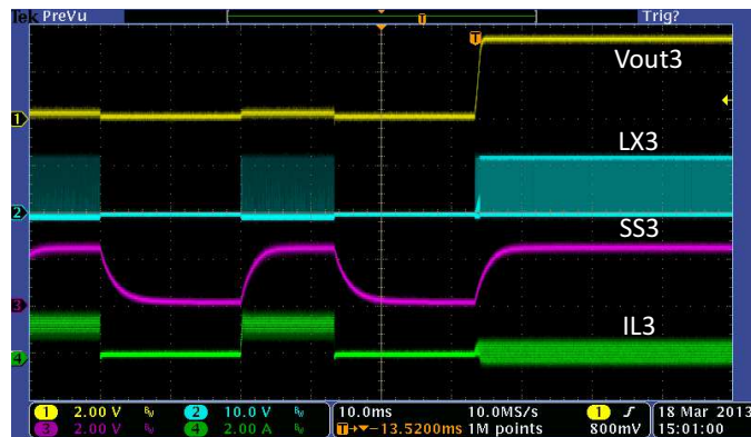
Figure 36. Hiccup Recover, Buck3=3.3V
