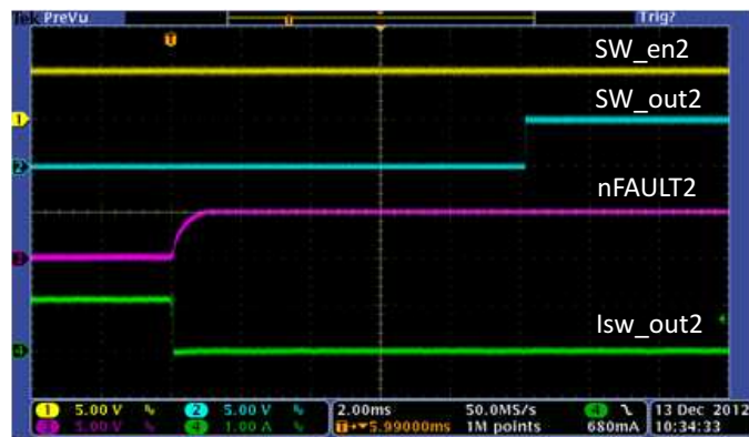
Figure 44. USB Switch2 Current Limit Recovery
