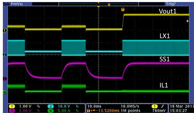
Figure 34. Hiccup Recover, Buck1=1.2V
