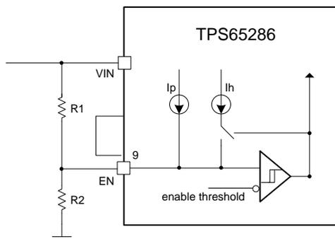
Figure 26. Adjustable VIN Under Voltage Lock Out
