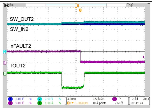
Figure 57. Power Switch2 Reverse Voltage Protection Response
