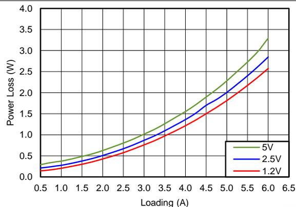
**Figure 59. Power Dissipation of TPS65286,
