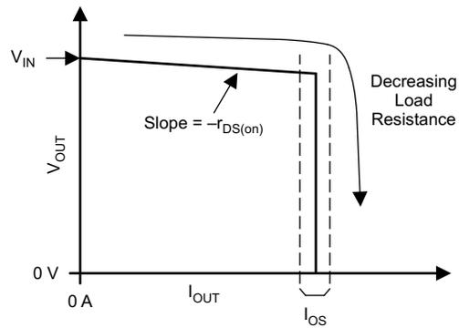
**Figure 3. Output Voltage vs Current Limit Threshold**
