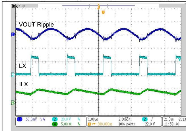
Figure 40. Buck Output Voltage Ripple,  $I_{OUT} = 4\text{ A}$
