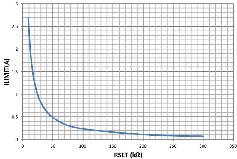
**Figure 23. Current-Limit Threshold I<sub>OS</sub> vs RLIM**
