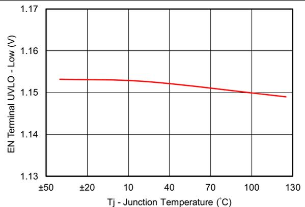
Figure 15. EN UVLO Stop vs Temperature
