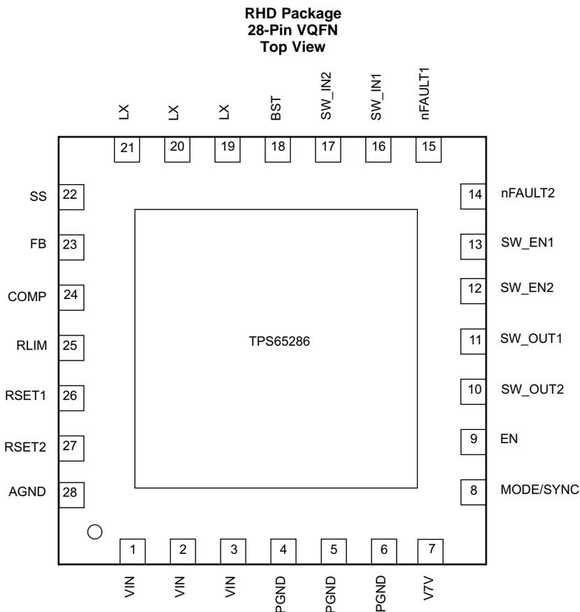
There is no electric signal down bonded to thermal pad inside IC. Exposed thermal pad must be soldered to PCB for optimal thermal performance.
