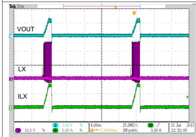
Figure 44. Buck Hiccup Response to Hard Short Circuit
