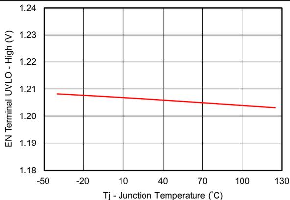
Figure 14. EN UVLO Start vs Temperature
