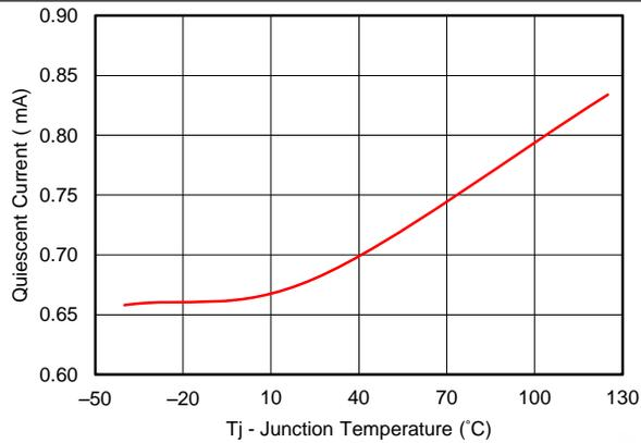
Figure 10. I<sub>IN</sub> (Without Switching) vs Temperature
