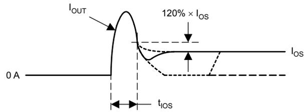
**Figure 2. Response Time to Short Circuit Waveform**
