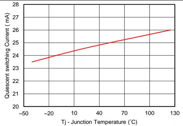
Figure 11. I<sub>IN</sub> (With Buck Switching) vs Temperature
