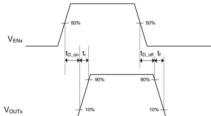
Figure 1. Power Switches Test Circuit and Voltage Waveforms
