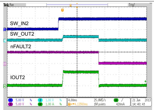
Figure 53. Power Switch2 Enable into Short Circuit
