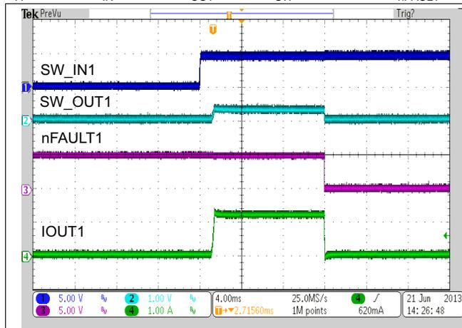
Figure 52. Power Switch1 Enable into Short Circuit
