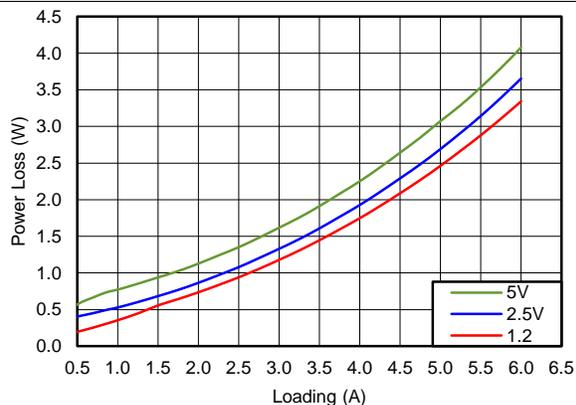
**Figure 58. Power Dissipation of TPS65286,
