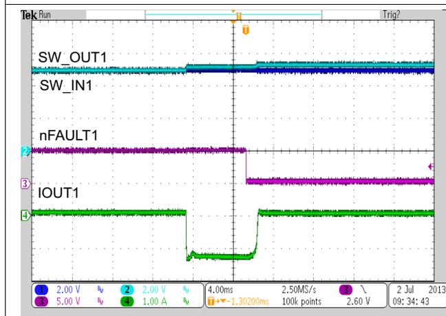
Figure 56. Power Switch1 Reverse Voltage Protection Response
