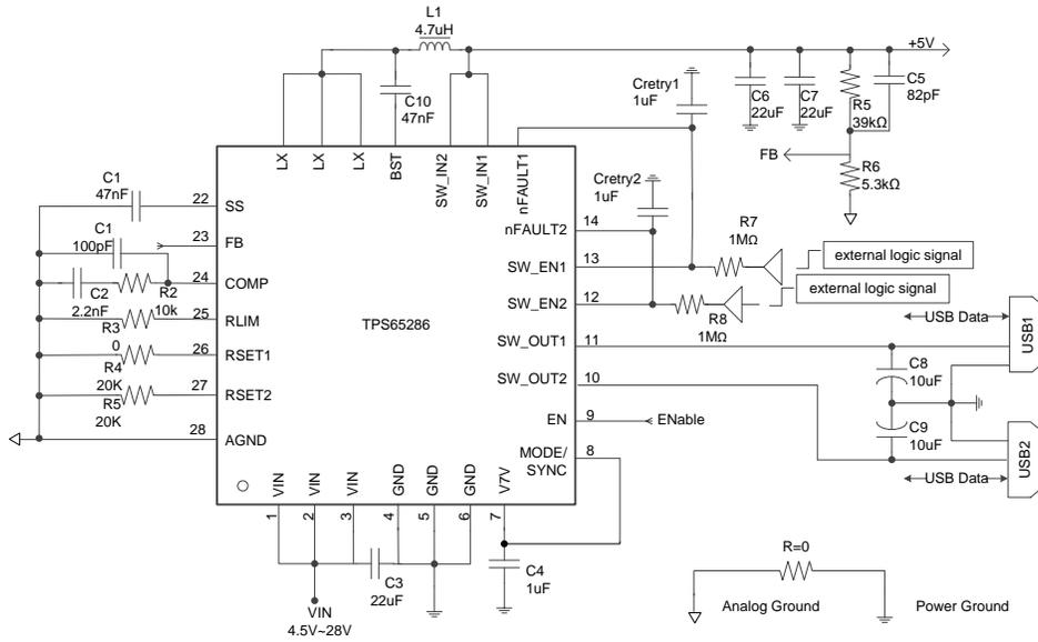
Figure 33. Auto Retry Functionality With External Enable Signal
