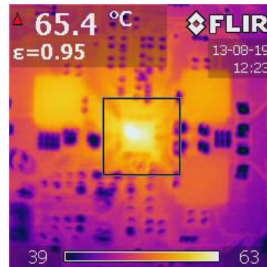
图 8-34. PWM Mode, Buck2, Steady State Operation with No Load
