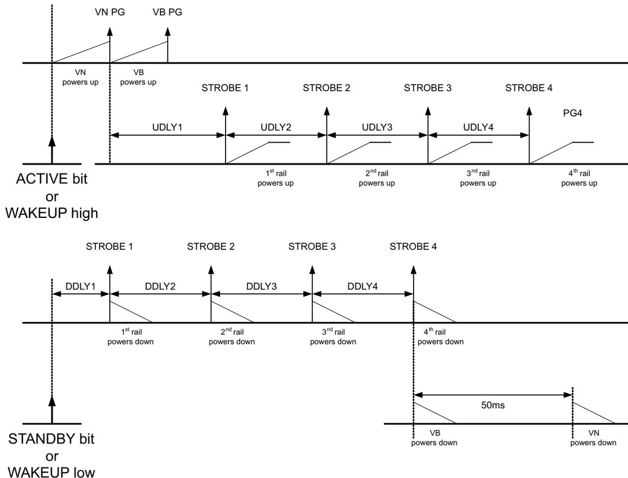
TOP: Power-up sequence is defined by assigning strobes to individual rails. STROBE1 is the first strobe to occur after ACTIVE bit is set and STROBE4 is the last event in the sequence. Strobes are assigned to rails in UPSEQ0 register and delays between STROBES are defined in UPSEQ1 register.
