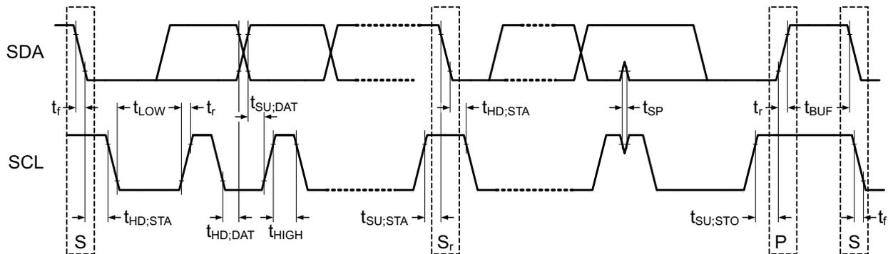
**Figure 1. I<sup>2</sup>C Data Transmission Timing**
