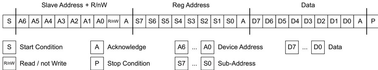
Figure 25. Subaddress in I<sup>2</sup>C Transmission
