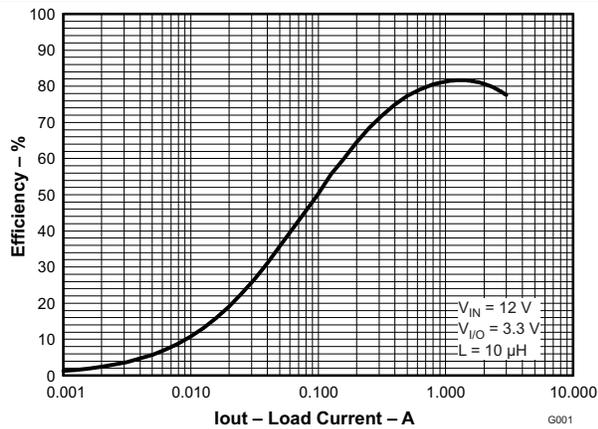
Figure 3. BUCK 1 ( $V_{I/O}$ ) EFFICIENCY vs LOAD CURRENT
