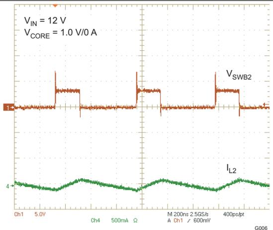
Figure 8. BUCK 2 ( $V_{CORE}$ ) PWM SWITCHING – LIGHT LOAD
