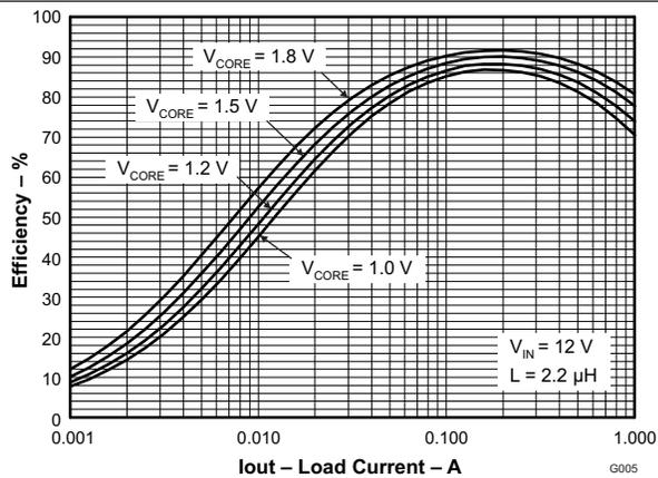
Figure 7. BUCK 2 ( $V_{CORE}$ ) EFFICIENCY vs LOAD CURRENT
