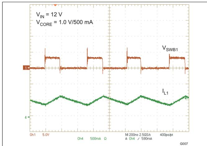
Figure 9. BUCK 2 (V<sub>CORE</sub>) PWM SWITCHING – HEAVY LOAD
