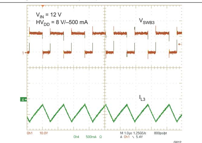
Figure 14. BUCK 3 (HV<sub>DD</sub>) PWM SWITCHING – HEAVY LOAD (SINK)
