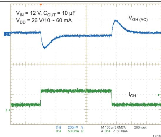
Figure 20. CPP (VGH) LOAD TRANSIENT RESPONSE
