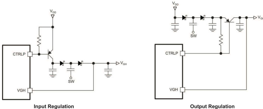
**Figure 25. Positive Charge Pump Application Circuits**
