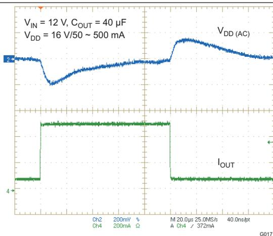
Figure 19. BOOST (VDD) LOAD TRANSIENT RESPONSE
