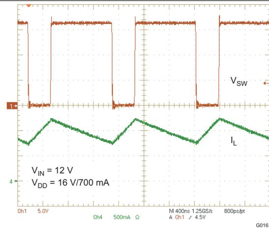
Figure 18. BOOST (VDD) PWM SWITCHING – HEAVY LOAD
