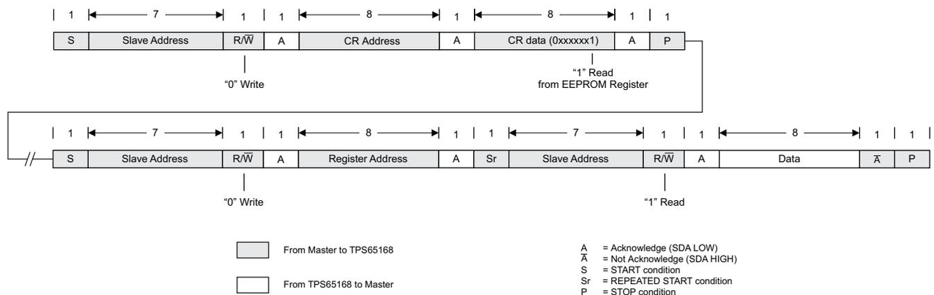
Figure 38. "Read" EEPROM Register Data Transfer Format
