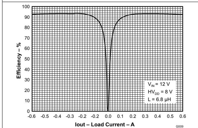
Figure 11. BUCK 3 (HV<sub>DD</sub>) EFFICIENCY vs LOAD CURRENT
