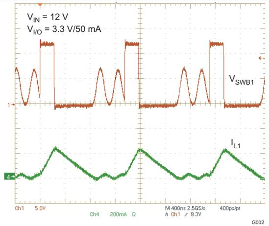
Figure 4. BUCK 1 ( $V_{I/O}$ ) PWM SWITCHING – LIGHT LOAD
