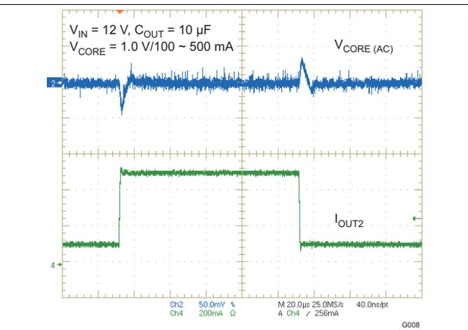
Figure 10. BUCK 2 (V<sub>CORE</sub>) LOAD TRANSIENT RESPONSE
