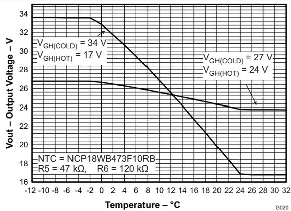
Figure 23. TEMPERATURE COMPENSATION VOLTAGE ADJUSTMENT
