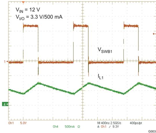
Figure 5. BUCK 1 ( $V_{I/O}$ ) PWM SWITCHING – HEAVY LOAD
