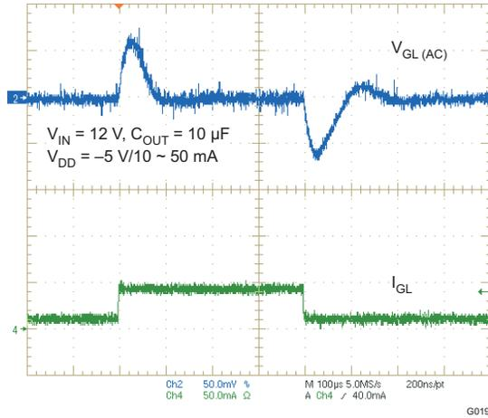
Figure 21. CPN ( $V_{GL}$ ) LOAD TRANSIENT RESPONSE
