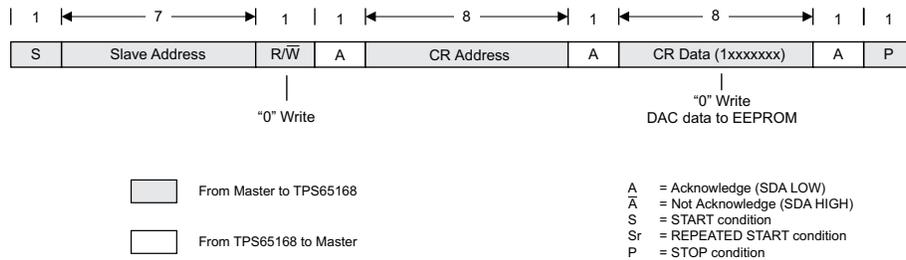
Figure 36. "Write" EEPROM Register Data Transfer Format
