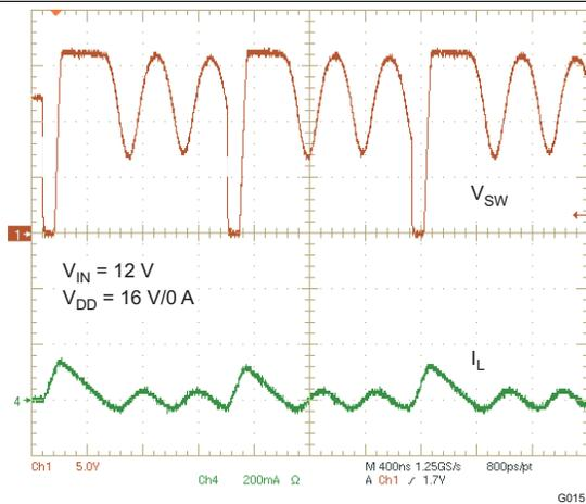
Figure 17. BOOST (VDD) PWM SWITCHING – LIGHT LOAD
