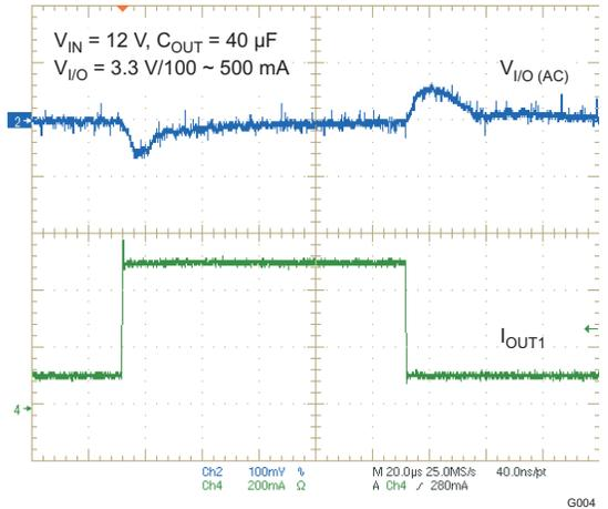
Figure 6. BUCK 1 ( $V_{I/O}$ ) LOAD TRANSIENT RESPONSE
