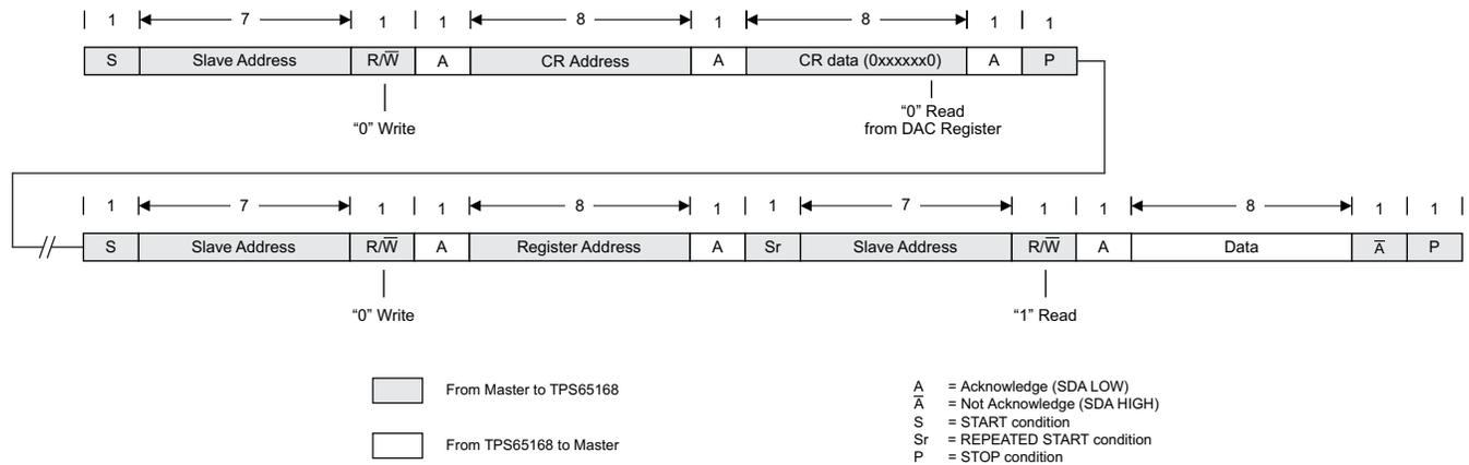
Figure 37. "Read" DAC Register Data Transfer Format
