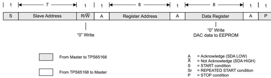
Figure 35. "Write" DAC Register Data Transfer Format
