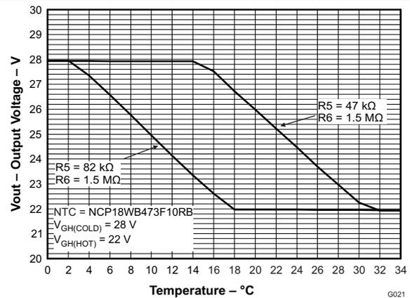
Figure 24. TEMPERATURE COMPENSATION TEMPERATURE ADJUSTMENT
