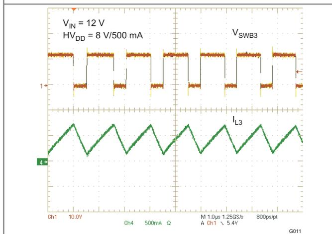
Figure 13. BUCK 3 (HV<sub>DD</sub>) PWM SWITCHING – HEAVY LOAD (SOURCE)
