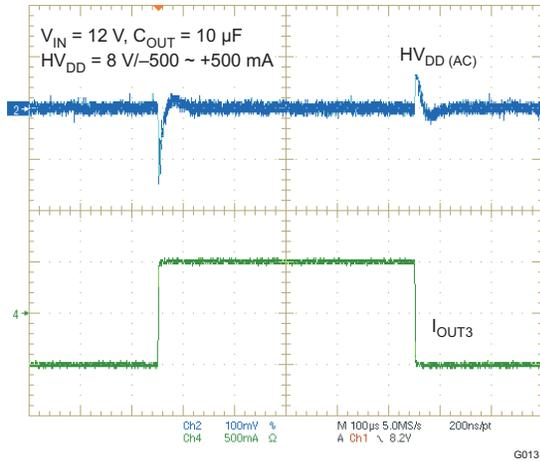
Figure 15. BUCK 3 (HVDD) LOAD TRANSIENT RESPONSE
