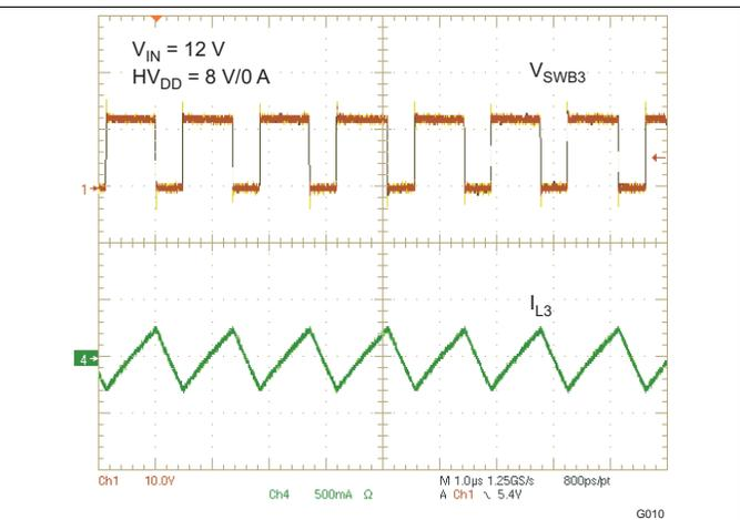
Figure 12. BUCK 3 (HV<sub>DD</sub>) PWM SWITCHING - LIGHT LOAD
