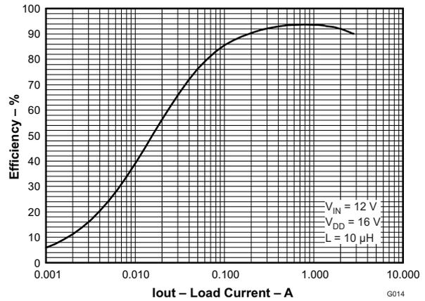
Figure 16. BOOST (VDD) EFFICIENCY vs LOAD CURRENT
