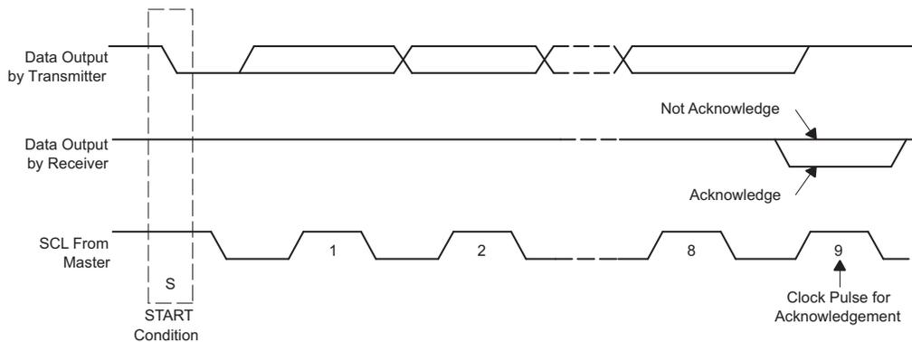
Figure 3-3. Acknowledge on the I<sup>2</sup>C-bus
