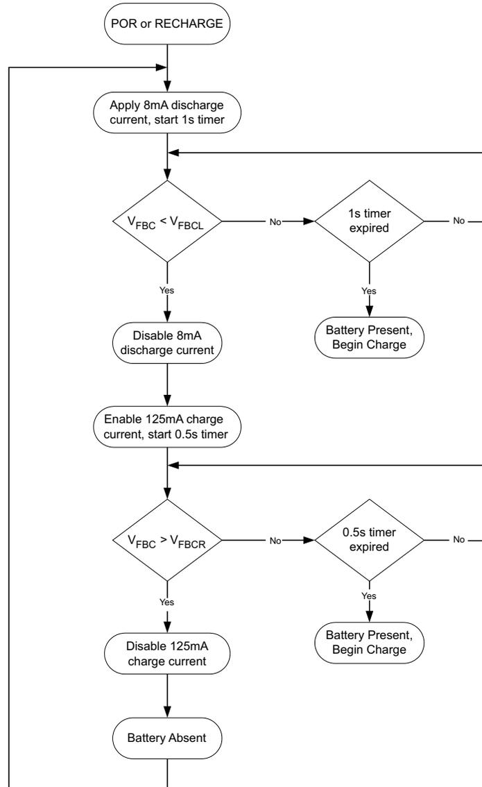
**Figure 3-7. Battery Detection**
