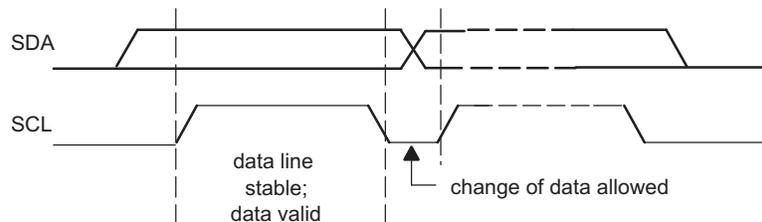
Figure 3-2. Bit Transfer on the I<sup>2</sup>C-bus
