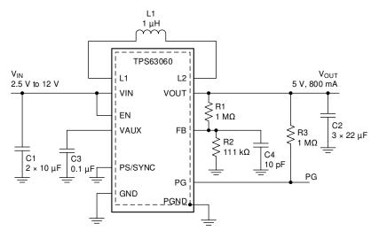
图 9-1. 5-V Adjustable Buck-Boost Converter Application
