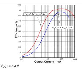
Figure 8. Efficiency vs Output Current – Power-Save Mode Disabled
