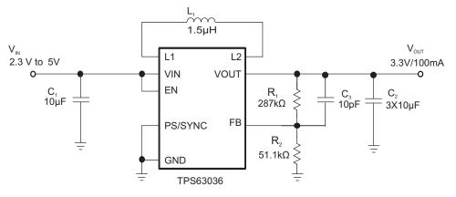
Figure 4. Typical Operating Circuit
