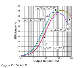
Figure 6. Efficiency vs Output Current – Power-Save Mode Disabled
