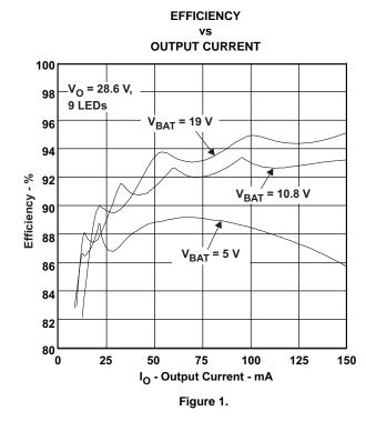
EFFICIENCY vs OUTPUT CURRENT
