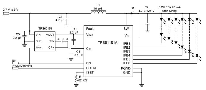
Figure 22. TPS61181A+TPS60151 for One Cell Li-ion Battery Power Application
