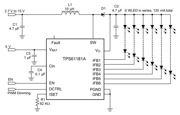
Figure 21. TPS61181A with Separate V<sub>BAT</sub> Power for Low Voltage Input Application
