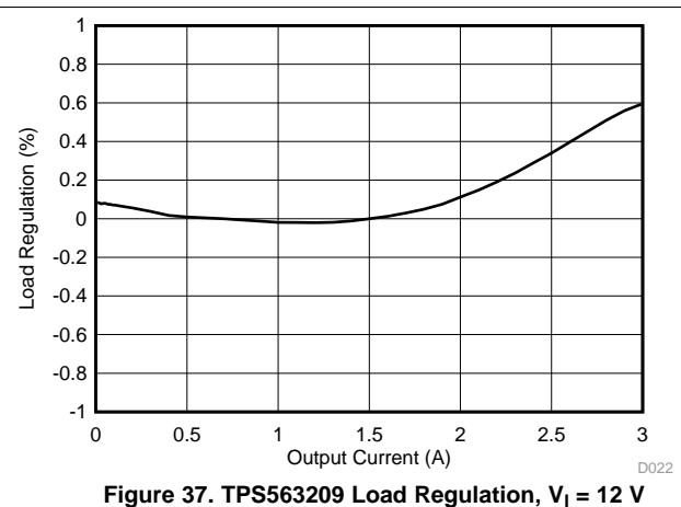
Figure 37. TPS563209 Load Regulation, V<sub>I</sub> = 12 V
