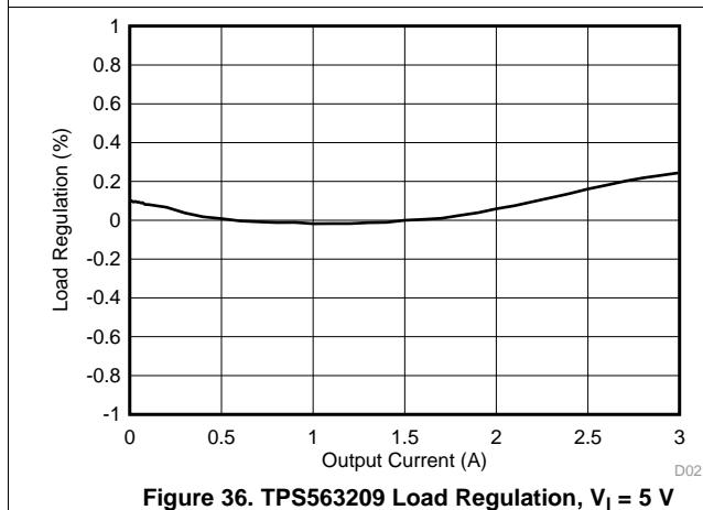
Figure 36. TPS563209 Load Regulation, V<sub>I</sub> = 5 V
