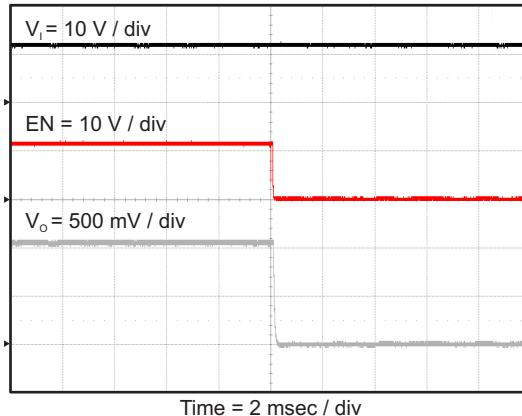
**Figure 32. TPS562209 Shut Down Relative to EN**
