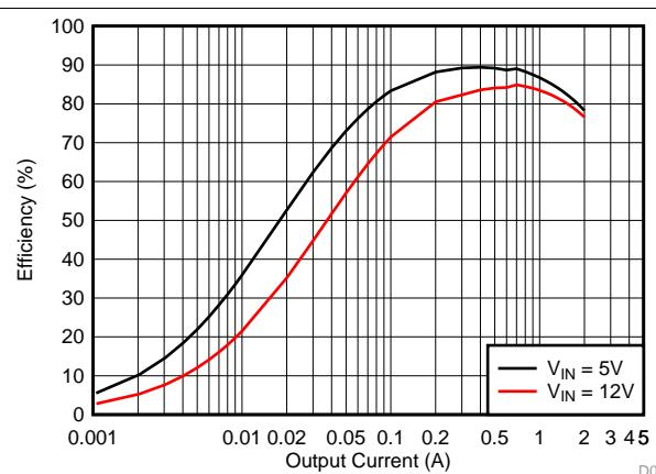
**Figure 22. TPS562209 Light Load Efficiency**
