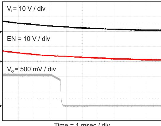
**Figure 44. TPS563209 Shut Down Relative to  $V_I$**
