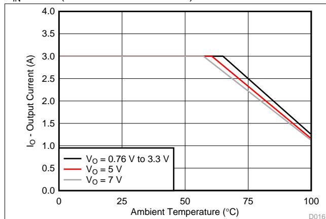
Figure 16. Output Current vs Ambient Temperature
