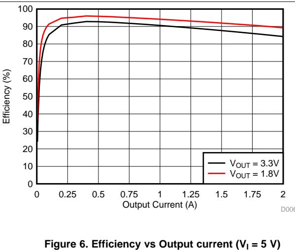
**Figure 6. Efficiency vs Output current ( $V_I = 5 V$ )**
