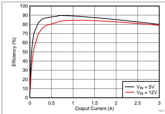
Figure 34. TPS563209 Efficiency
