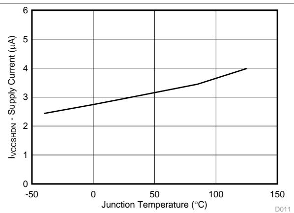
**Figure 11. VIN Shutdown Current vs Junction Temperature**
