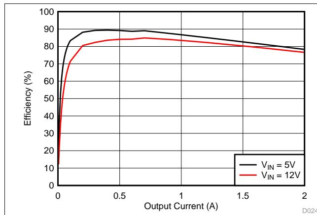
**Figure 21. TPS562209 Efficiency**
