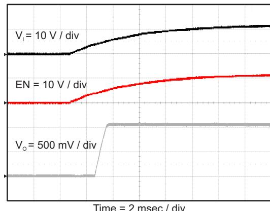
**Figure 29. TPS562209 Start Up Relative to  $V_i$**
