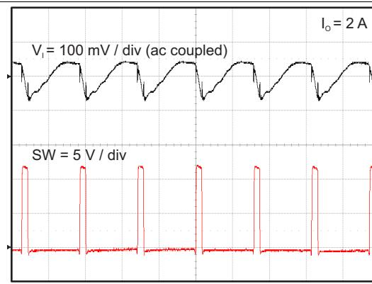
**Figure 26. TPS562209 Input Voltage Ripple**
