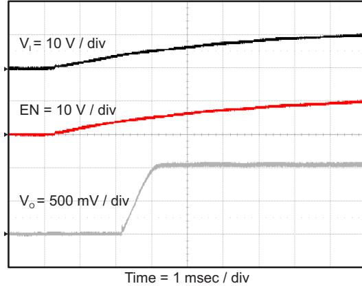
Figure 42. TPS563209 Start Up Relative to V<sub>i</sub>
