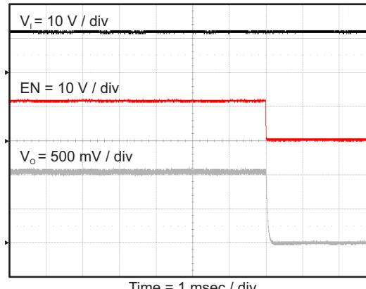
**Figure 45. TPS563209 Shut Down Relative to EN**
