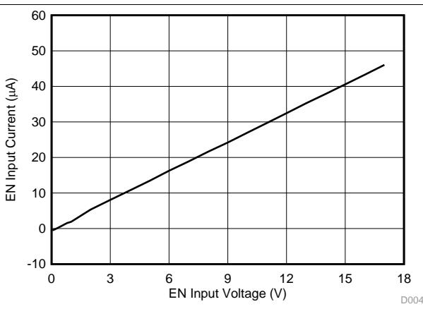
**Figure 4. EN Current vs EN Voltage**
