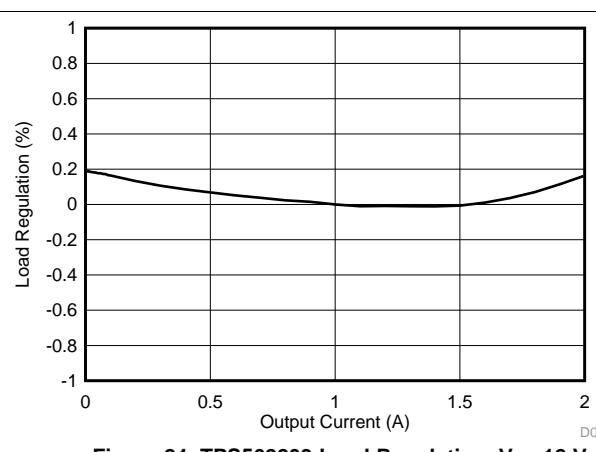
**Figure 24. TPS562209 Load Regulation,  $V_I = 12\text{ V}$**
