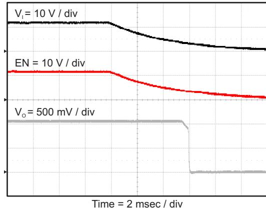
**Figure 31. TPS562209 Shut Down Relative to  $V_i$**
