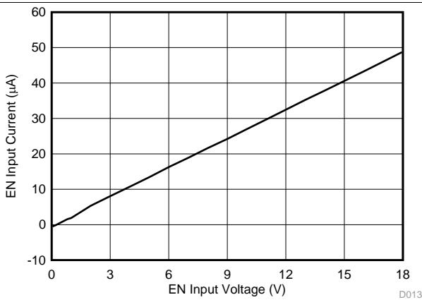
**Figure 13. EN Current vs EN Voltage**
