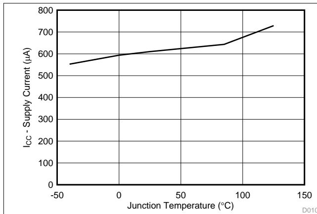
**Figure 10. Supply Current vs Junction Temperature**
