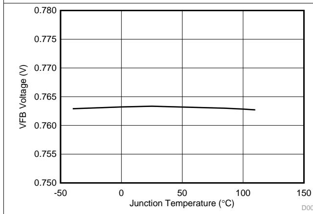
**Figure 3. VFB Voltage vs Junction Temperature**
