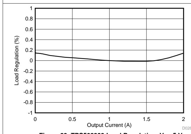
**Figure 23. TPS562209 Load Regulation,  $V_I = 5\text{ V}$**
