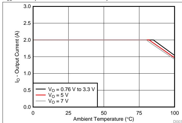
Figure 7. Output Current vs Ambient Temperature
