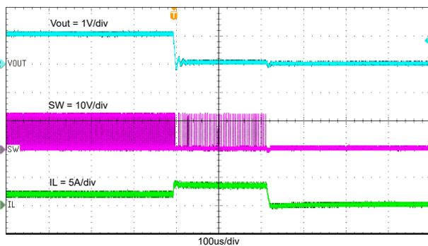
图 8-14. Normal Operation to Output Hard Short
