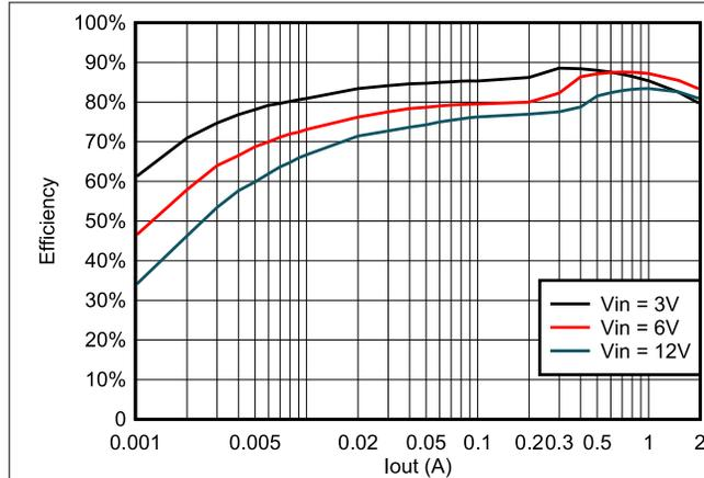
图 6-7. Efficiency at 0.8  $V_{OUT}$  with a 1- $\mu\text{H}$  Inductor
