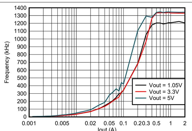
图 6-12. Frequency vs Loading,  $V_{IN} = 12\text{ V}$
