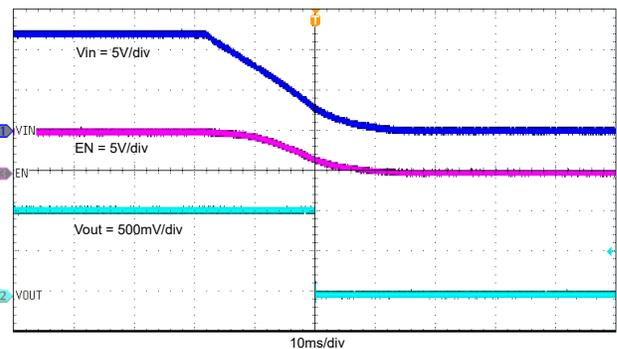
图 8-11. Shutdown with  $V_{IN}$  Falling,  $I_{OUT} = 2\text{ A}$
