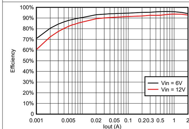
图 6-9. Efficiency at 3.3  $V_{OUT}$  with a 2.2- $\mu\text{H}$  Inductor
