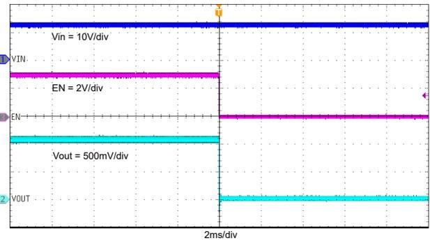
图 8-9. Shutdown Through EN,  $I_{OUT} = 2\text{ A}$
