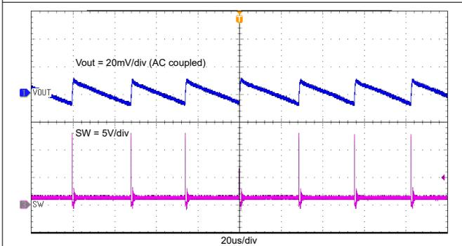
图 8-6. Output Voltage Ripple with 0.01-A Loading
