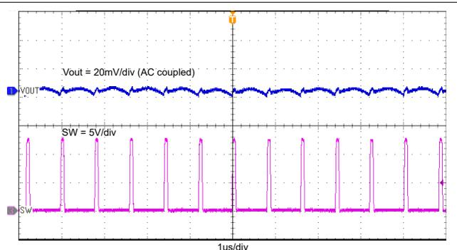
图 8-7. Output Voltage Ripple with 2-A Loading
