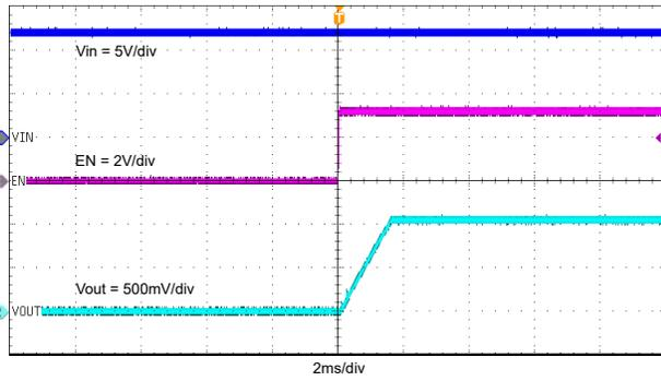
图 8-8. Start-up Through EN,  $I_{OUT} = 2\text{ A}$
