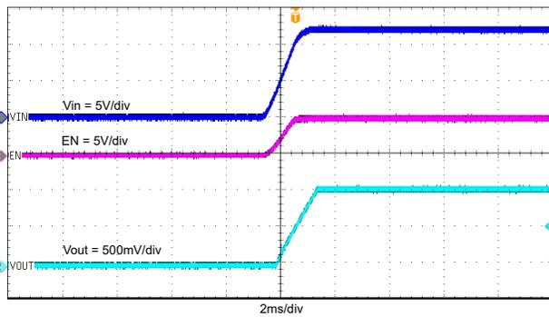
图 8-10. Start-up with  $V_{IN}$  Rising,  $I_{OUT} = 2\text{ A}$
