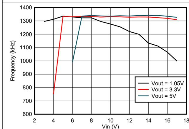
图 6-11. Frequency vs Input Voltage,  $I_{OUT} = 2\text{ A}$
