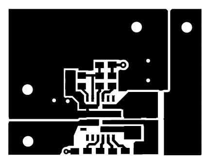
图 64. Top Layer of Example Converter Layout
