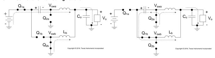
图 44. Phase A High Side MOSFET On
