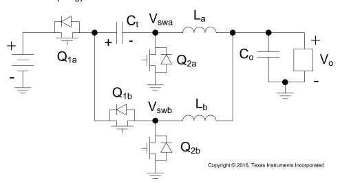
图 43. Two-Phase Series Capacitor Buck Converter Topology
