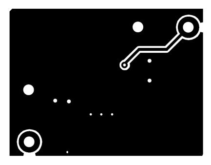
图 65. Bottom Layer of Example Converter Layout
