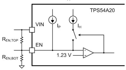
图 42. Adjustable VIN Undervoltage Lockout
