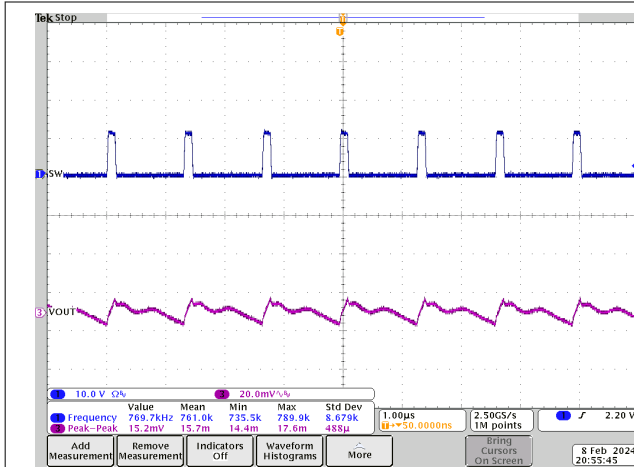
图 7-14. 输出电压纹波, 800kHz FCCM, 40A 负载, PVIN = 12V, VOUT = 1.1V
