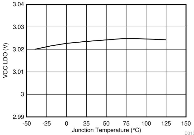
$V_{IN} = 12V$   $I_{VCC} = 2 mA$
