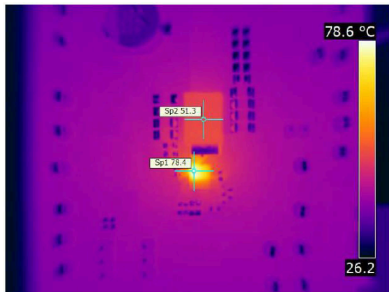
图 6-13. Thermal Image at 15-A Output Current
