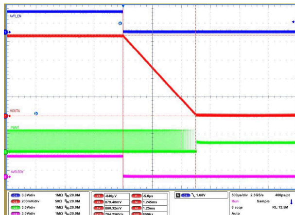
图 8-9. Soft-stop channel A (0 ms TOFF_DELAY)
