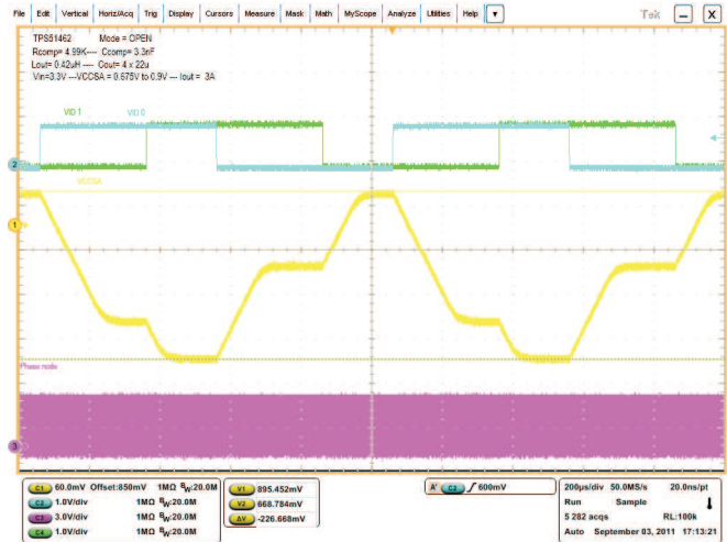
Figure 15. Mode=8, I_{OUT} = 3 A, VID Transitioning
